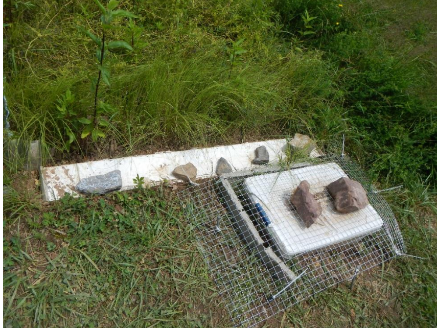
Figure 70: CH-3 WVDOH type B (TS, HP, 1) collection gutter and storage container with rolled wire reinforcement
