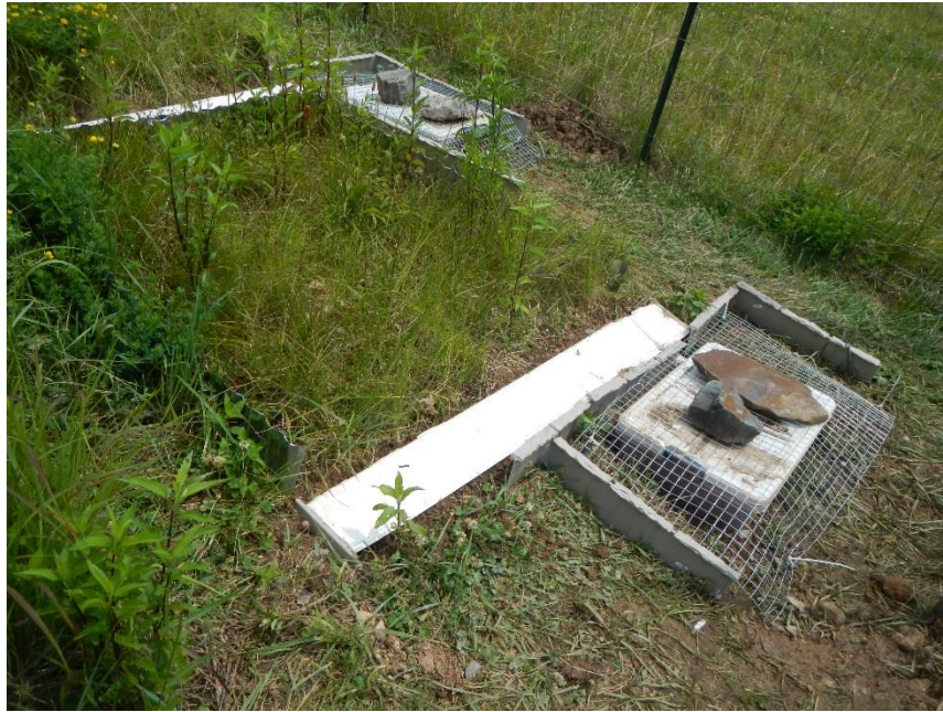
Figure 71: CH-3 WVDOH type B (NTS, S, 2) and (TS, S, 2) left view of sedimentation collection apparatuses
