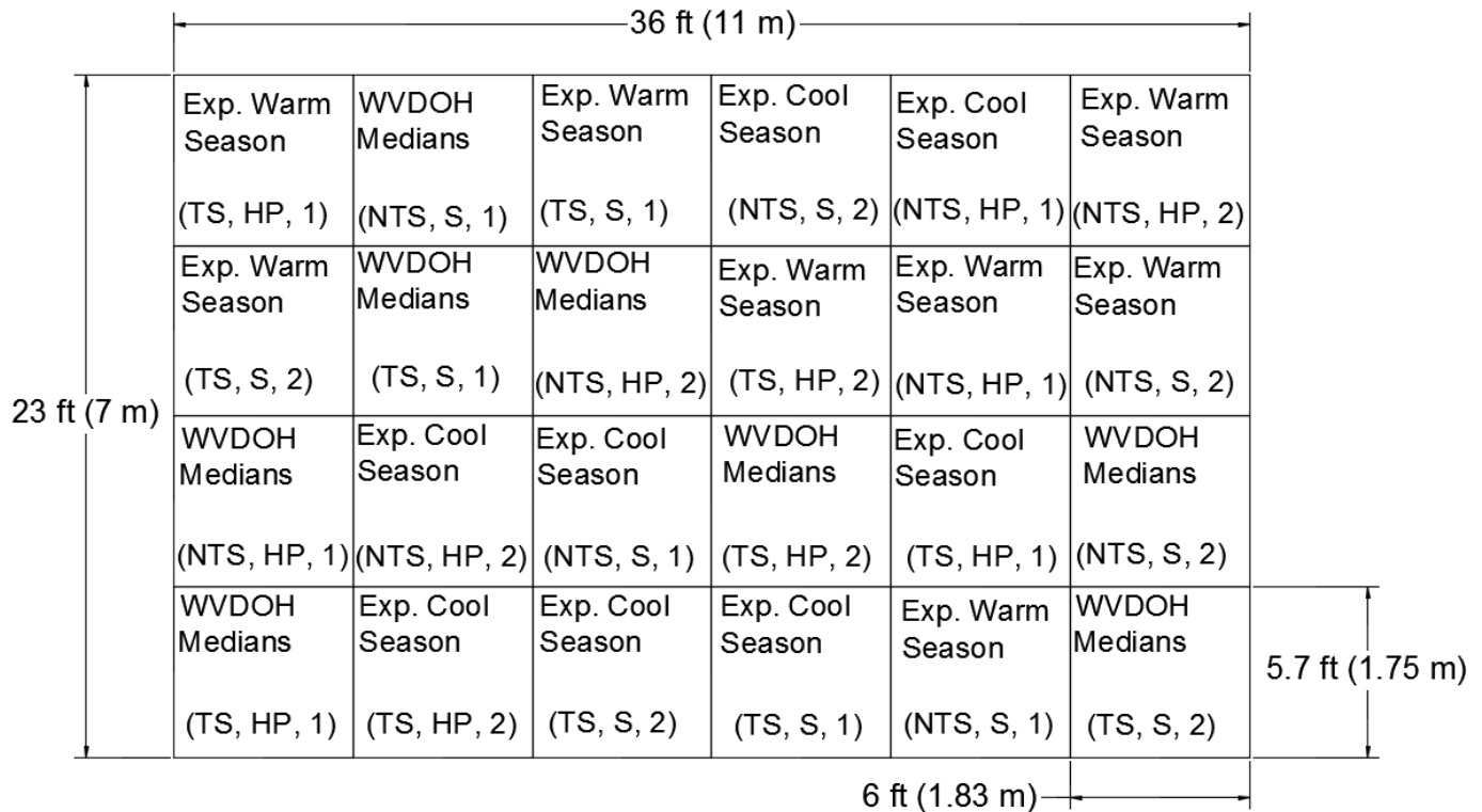
Figure 3: CH-3 subplot layout (TS=topsoil; NTS=no Topsoil; S=straw Mulch; HP=hydraulic erosion control product)
