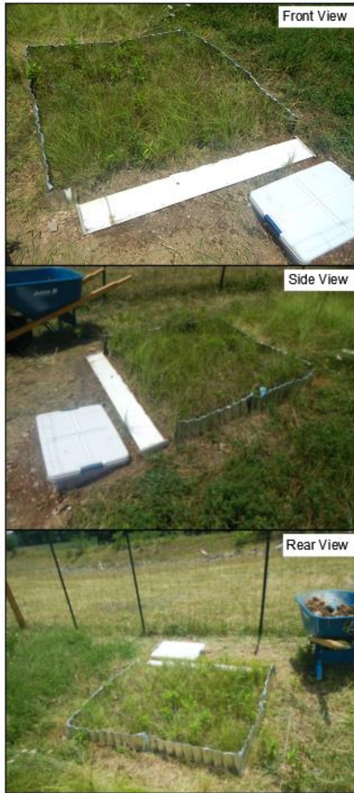
Figure 68: All angle views of trial sedimentation and runoff apparatus
