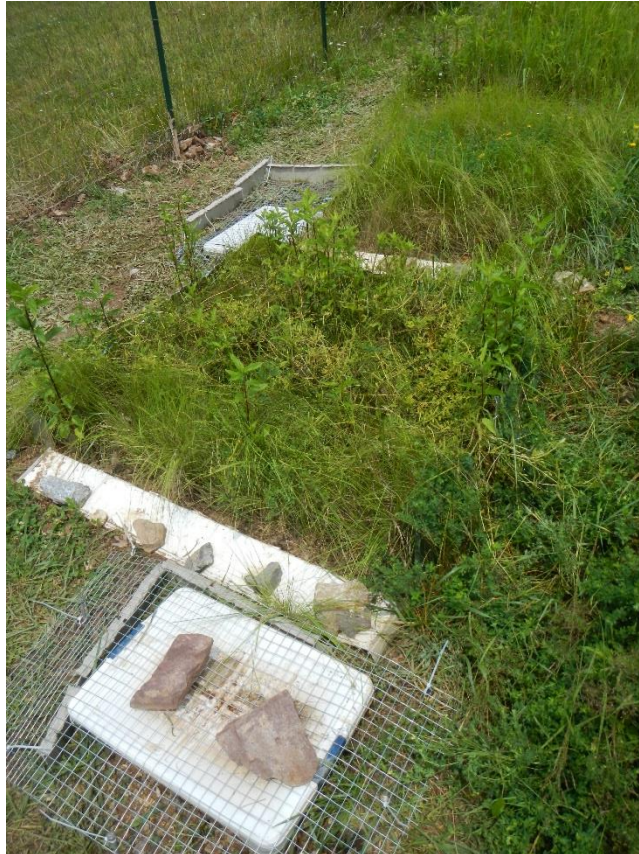
Figure 69: CH-3 WVDOH type B (NTS, HP, 1) and (TS, HP, 1) front view of sedimentation collection apparatuses
