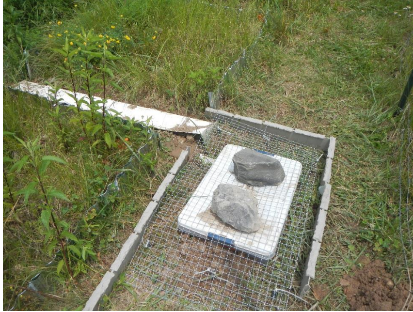
Figure 72: CH-3 WVDOH type B (NTS, S, 2) sediment and runoff collection apparatus
