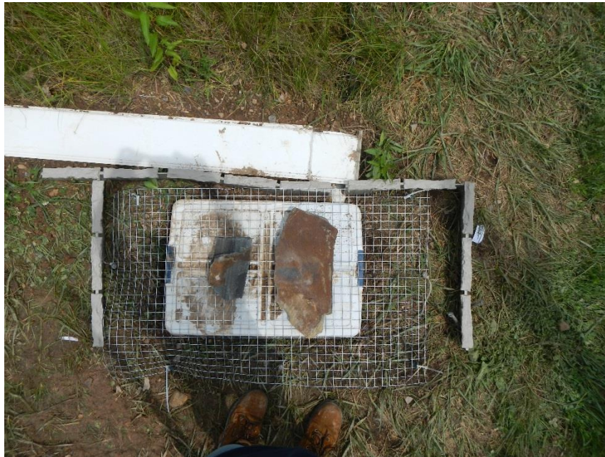
Figure 73: CH-3 WVDOH type B (TS, S, 2) sediment and runoff collection apparatus
