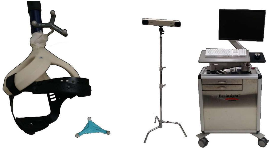
Figure 19: The hardware used for neuronavigation. On left, the subject array and coil array, affixed to the coil. On right, the Polaris camera and Rogue Research/Brainsight computer station.
