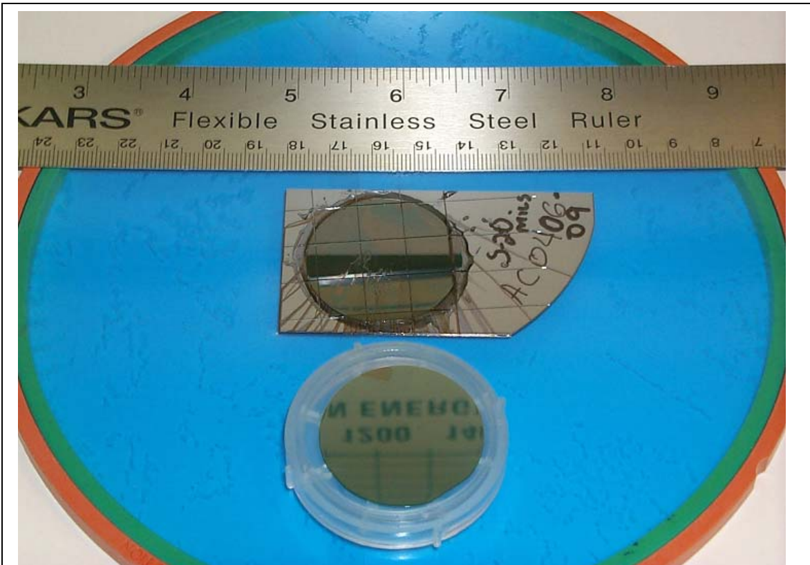
Figure 3.14. Image of a diced and un-diced CREE Inc. 1" 6H-SiC wafer.
