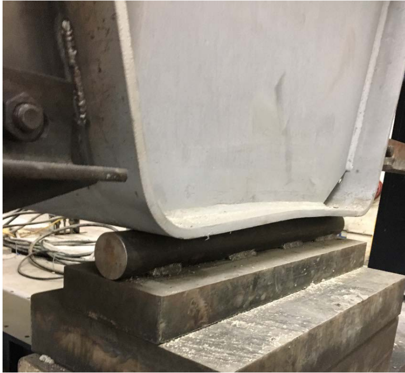
Figure 4.3: View of Pinned Boundary Condition
