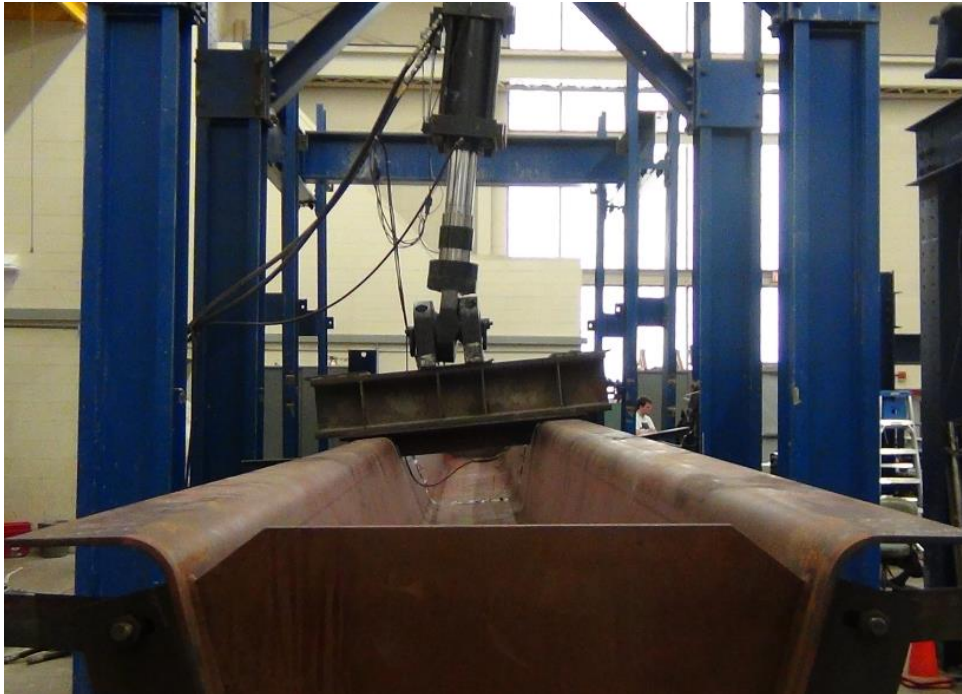
Figure 2.13: Lateral Torsional Buckling (Kelly, 2014)
