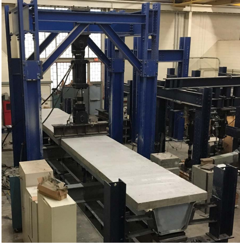
Figure 4.17: Load Applied to the System
