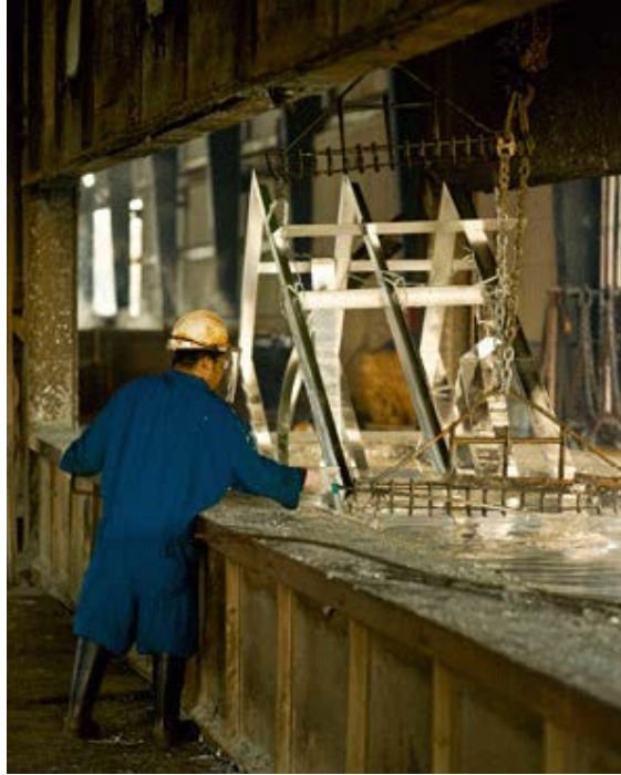
Figure 2.23: Dipping of Steel in Molten Zinc (American Galvanizers Association, 2018)
