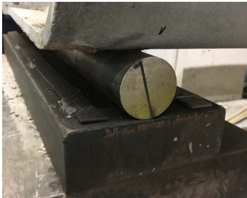
Figure 4.4: View of Roller Boundary Condition
