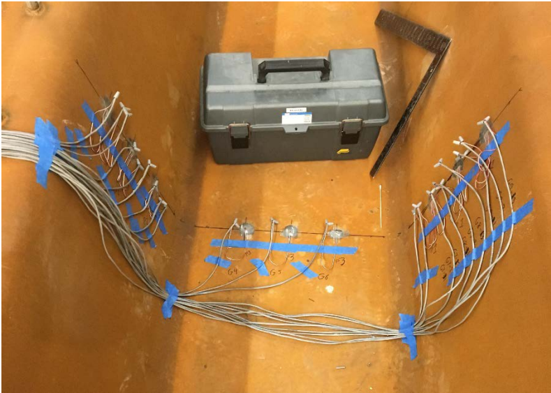
Figure 4.10: Exposed Strain Gages
