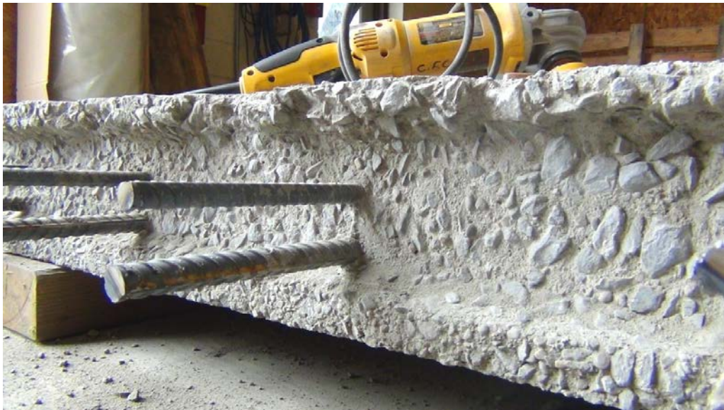
Figure 2.14: Concrete Surface after Wire-Brushing (Kozhokin, 2016)
