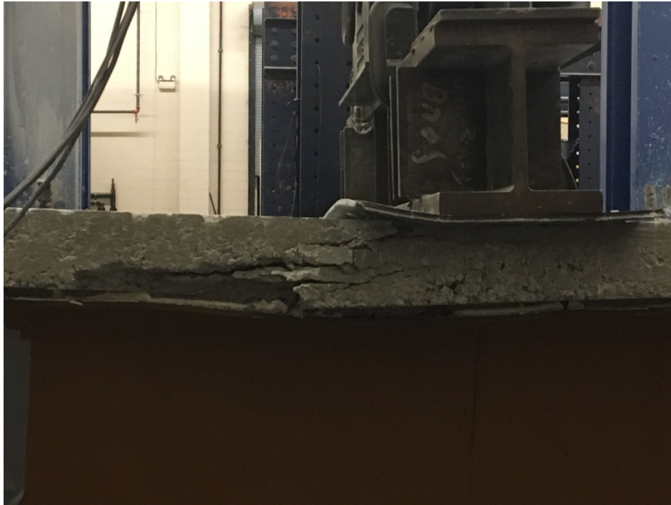
Figure 4.18: Typical Failure Mode for Composite Specimens
