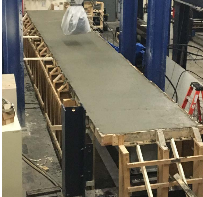
Figure 4.16: Poured Concrete Deck
