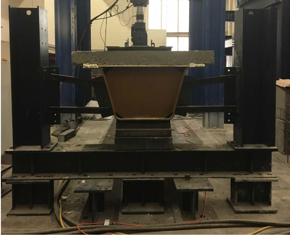
Figure 4.5: Lateral Bracing System
