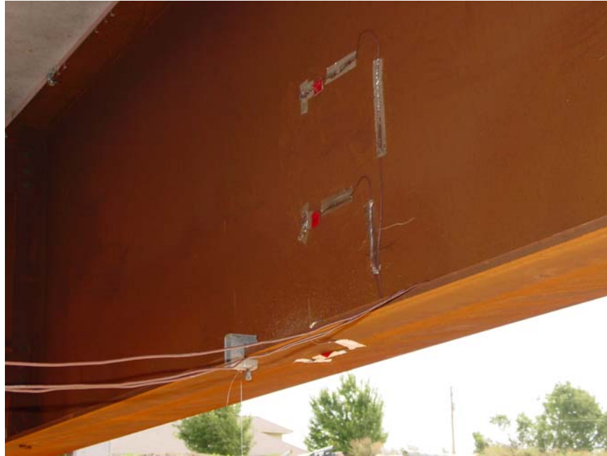
Figure 7.8. Strain gages for one exterior girder
