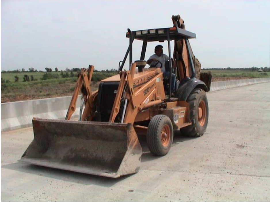
Figure 7.18. Construction vehicle used for dynamic testing
