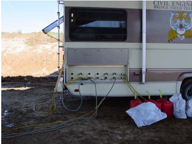
Figure 7.6. Data acquisition connector panel
