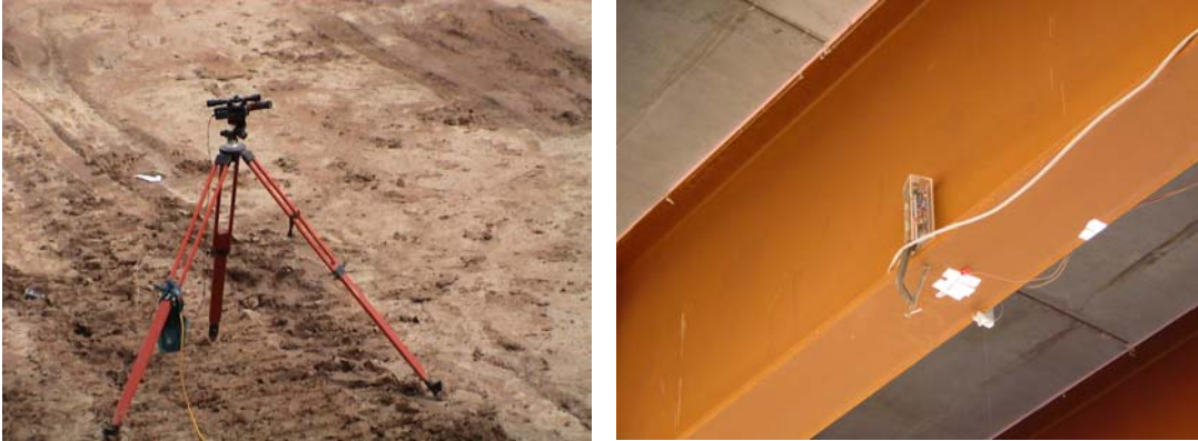
Figure 7.10. Laser deflection devices
