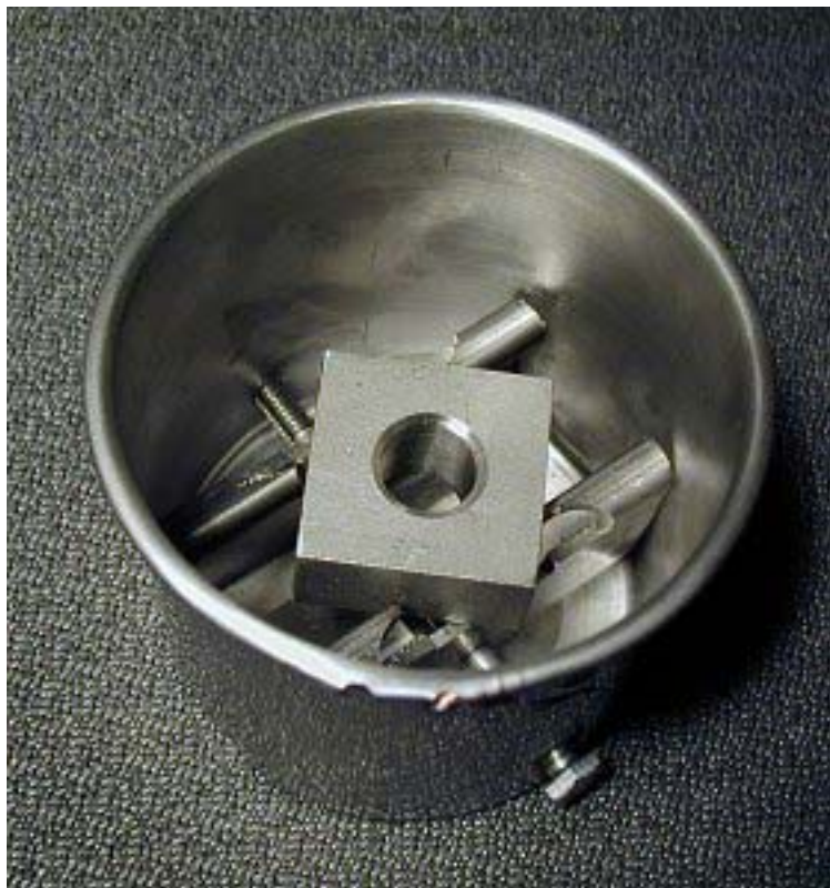
Figure 2.19: Stainless Steel Strut Channel and Seat Bolted into Specimen Cup
