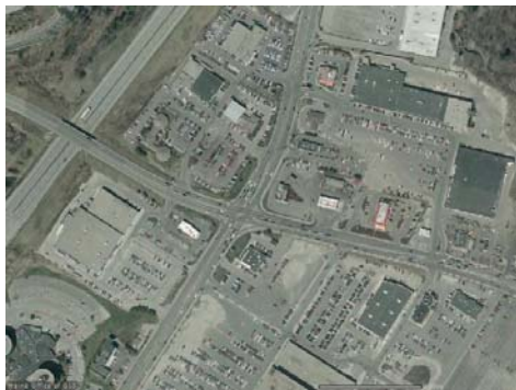
Nearly a third of the Long Creek watershed is covered by impervious surfaces like roofs and parking lots. To combat stormwater pollution in the Creek, CBEP helped develop a watershed management plan.
