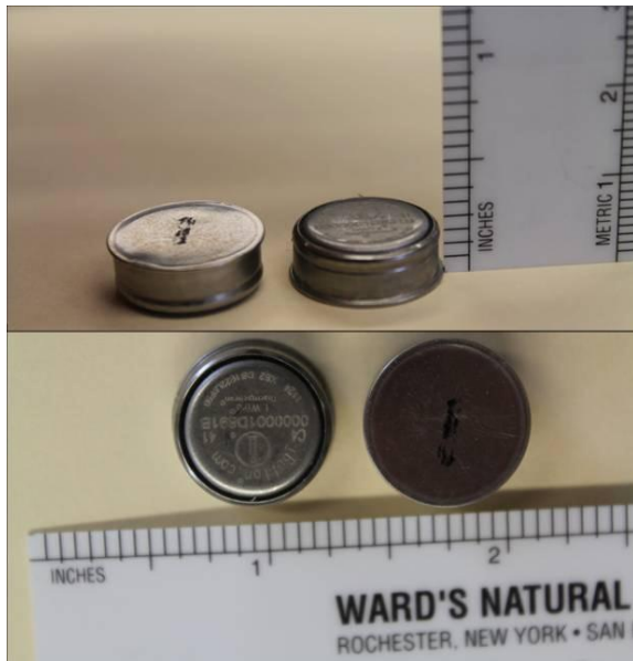
Figure 13: ThermoChron iButton model DS1922L. Twenty-one iButtons were attached to wooden dowels and installed in the streambed. They logged temperatures at 15 -minute intervals from 18 February to 26 March, 2012
