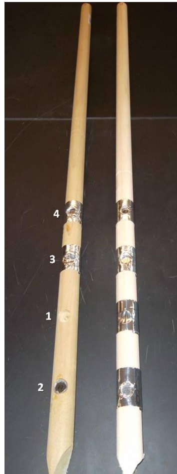
Figure 14: iButton dowel construction. The left dowel shows each stage of construction. 1) Hole drilled in 3.18 cm diameter wooden dowel (second from bottom), 2) iButton sealed in the hole (bottom), 3) iButton covered with waterproof tape (second from top), 4) Hole cut in waterproof tape to expose the face of the iButton (top). The dowel on the right shows a complete dowel construction. Four holes were drilled on each dowel, but iButtons were installed in only three holes.
