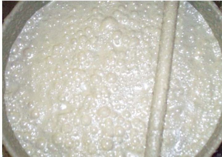
Figure 4.05: Observation of Air Bubbles coming to the Surface of Static Mix.
