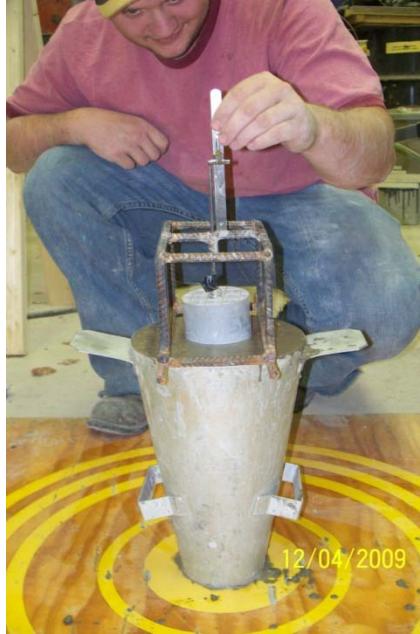
Figure 2.03: Picture of Performing the Measurement of Probe Depth.
