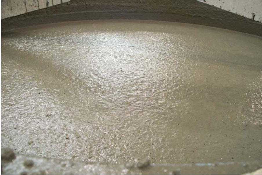
Figure 4.02: Air Bubbles Escaping from a Freshly Batched SCC During a Trial Mix.
