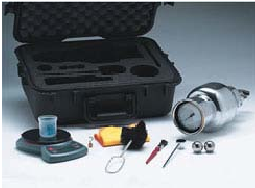
Figure 2.01: Speedy Moisture Meter Setup.
