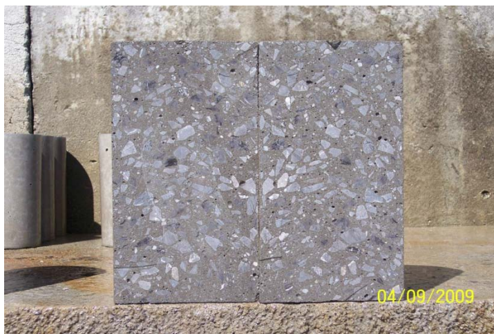
Figure 1.03: Prepared Sample for the Hardened VSI Test.
