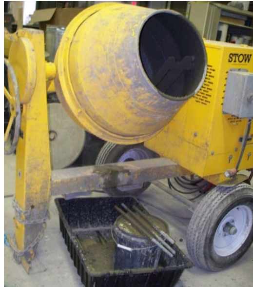
Figure 4.03: Batching of SCC Mix for the Observation of Air Migration.
