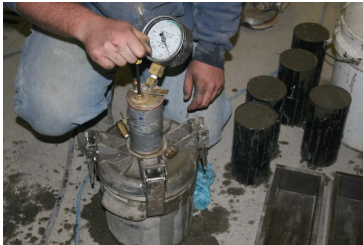
Figure 1.02: Air Content Test using Type B Pressure Meter.
