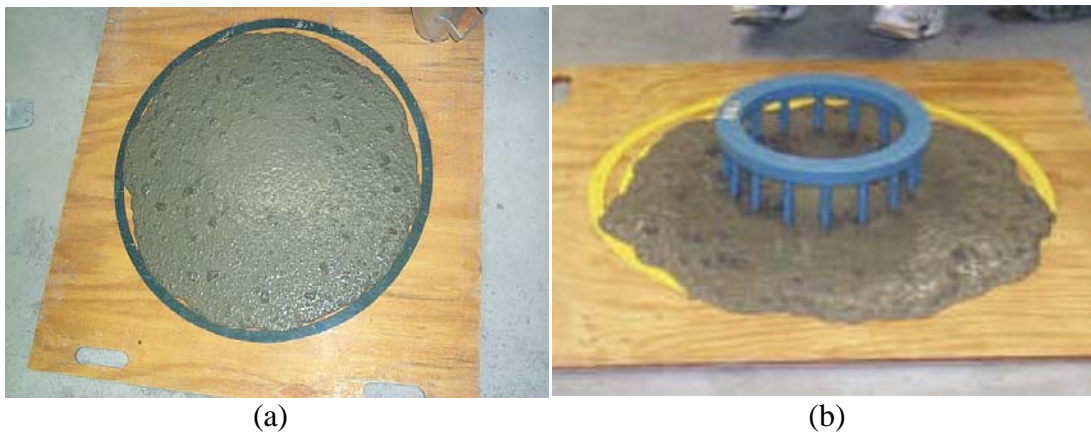
Figure 1.01: (a) Picture of the Fresh Concrete Patty after the Slump Flow Test for SCC. (b) Picture of the Fresh Concrete Patty after the J-Ring Test for SCC.
