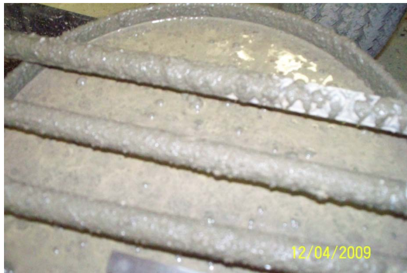
Figure 4.04: Few Air Bubbles Rising to the Surface upon First Batch.
