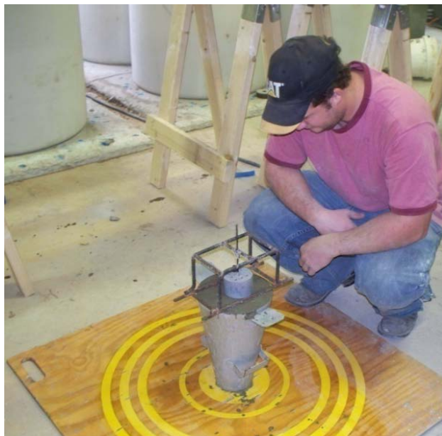
Figure 2.02: Picture of Performing the Segregation Probe Test on an SCC Mix.
