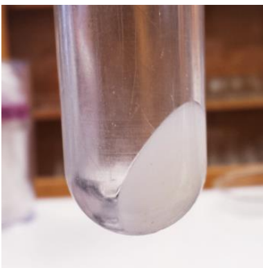
Figure 3.13 The pellet containing polymerized LMM and undigested myosin. The white pellet on the bottom of the centrifuge container is a mixture of polymerized LMM and undigested myosin.
