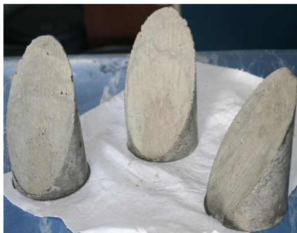
Figure 6.25 Substrate concrete (NC)
