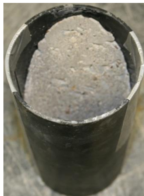
Figure 6.27 Mold ready for repair casting
