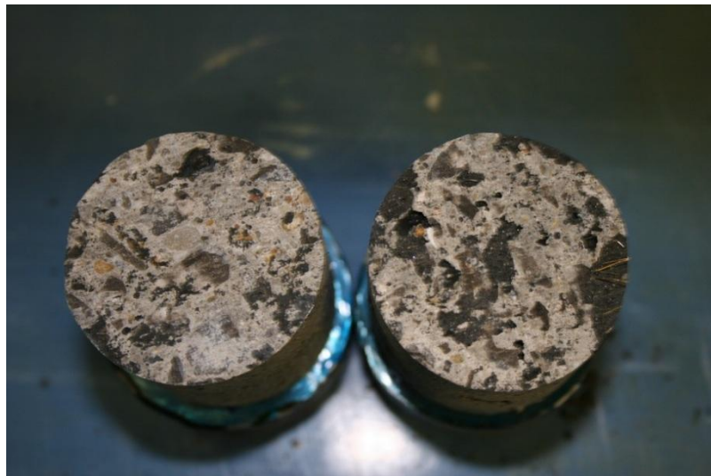
Figure 6.46 Failure through substrate (pull-off)
