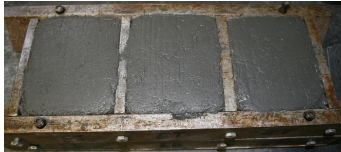
Figure 6.8 Finished surface of repair material (HPFRC)
