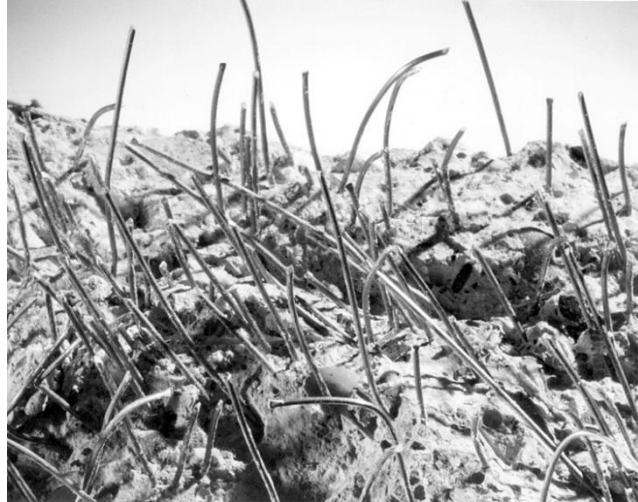
Figure 2.5 Fracture surface of SFRC (from ACI 544.1R)
