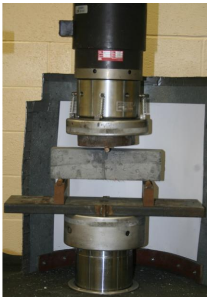
Figure 5.7 Test setup for flexure specimens
