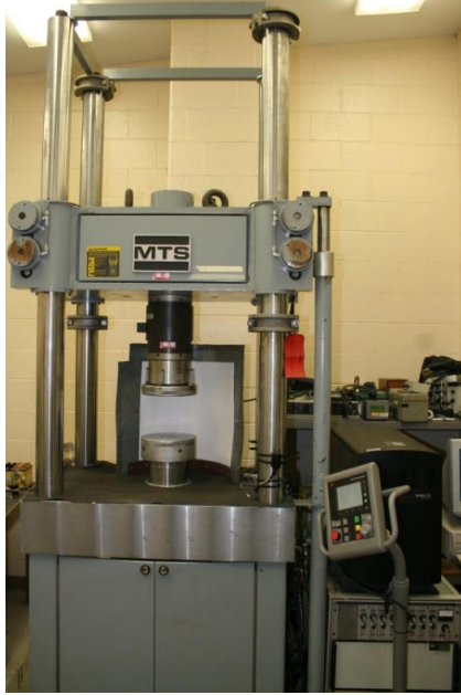
Figure 5.2 MTS machine used for compressive strength test
