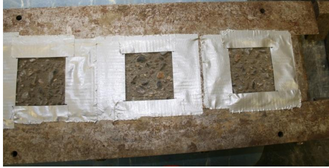
Figure 6.6 Reduced bond area
