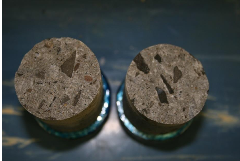
Figure 6.46 Failure through substrate (pull-off)
