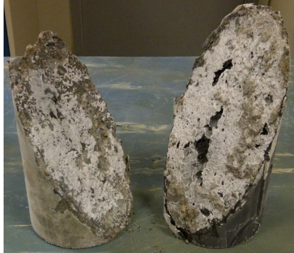
Figure 6.30 Failure through interface
