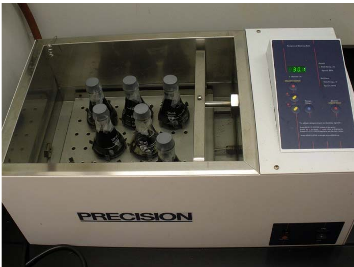
Figure 3.3 Experimental setup showing shaker bath with sample flasks
