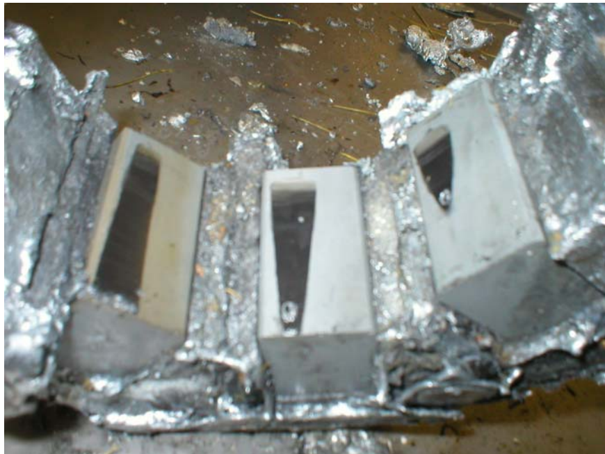
Figure 25 Wearing on Ceramic Insert after Cycle 2 (13 hr & 45 min)
