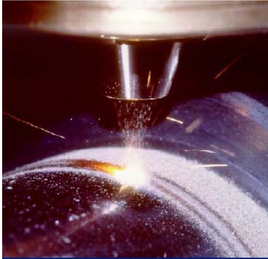
Figure 2 Tungsten Carbide Composite is Metallurgically Bonded by a Laser Process to a 316L Stainless Steel Sleeve [1]
