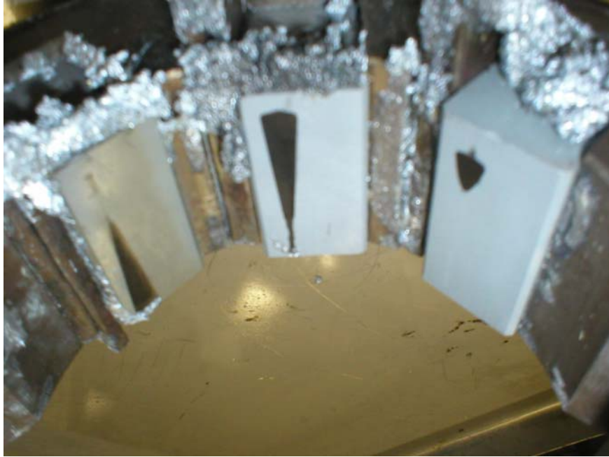
Figure 24 Wearing on Ceramic Insert after Cycle 1 (6 hr & 15 min)
