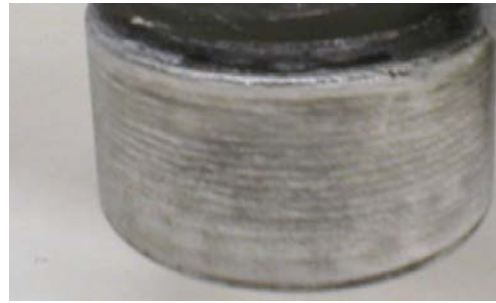
Figure 10 CF3M Coated with Tungsten Carbide by Laser Cladding process
