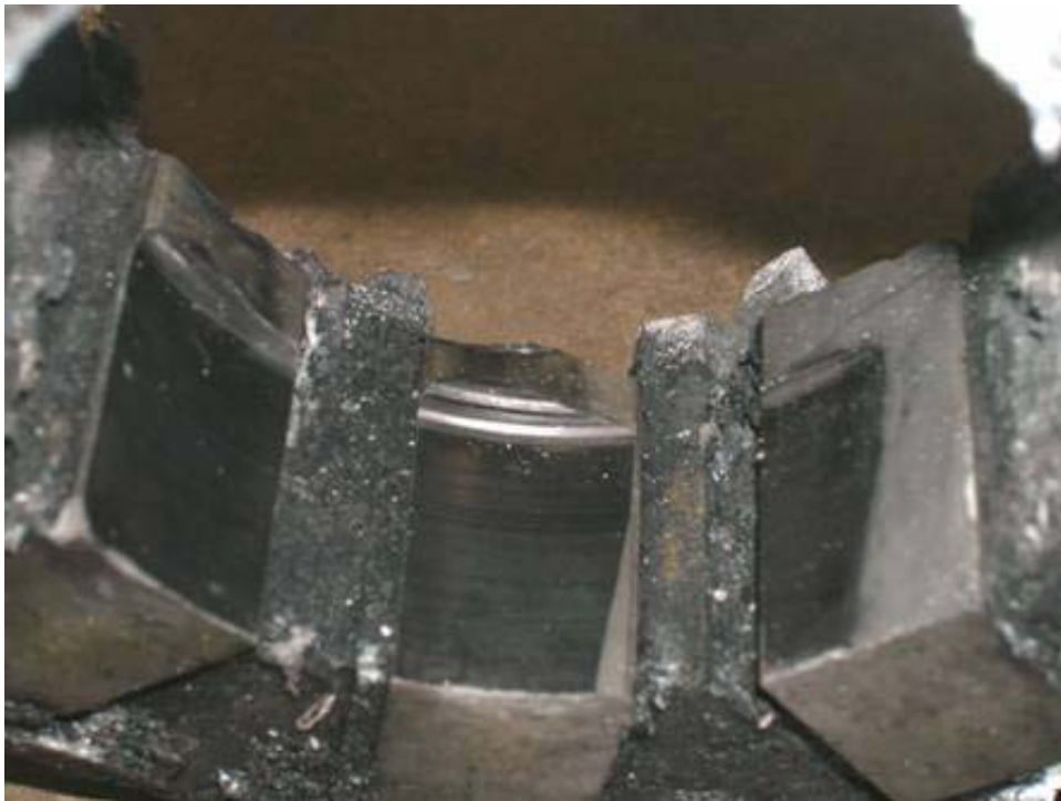
Figure 39 Wearing on Ceramic Insert after Cycle 5 (3 hrs at 50% Production Line Tension)
