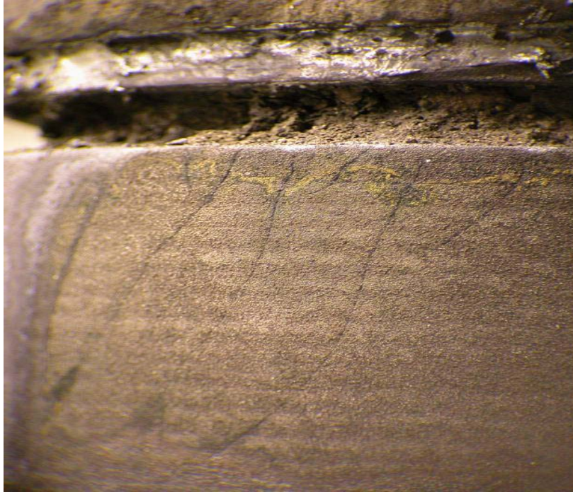
Figure 41 Cracks on the Wearing Sleeve Surface after Test Cycle 2
