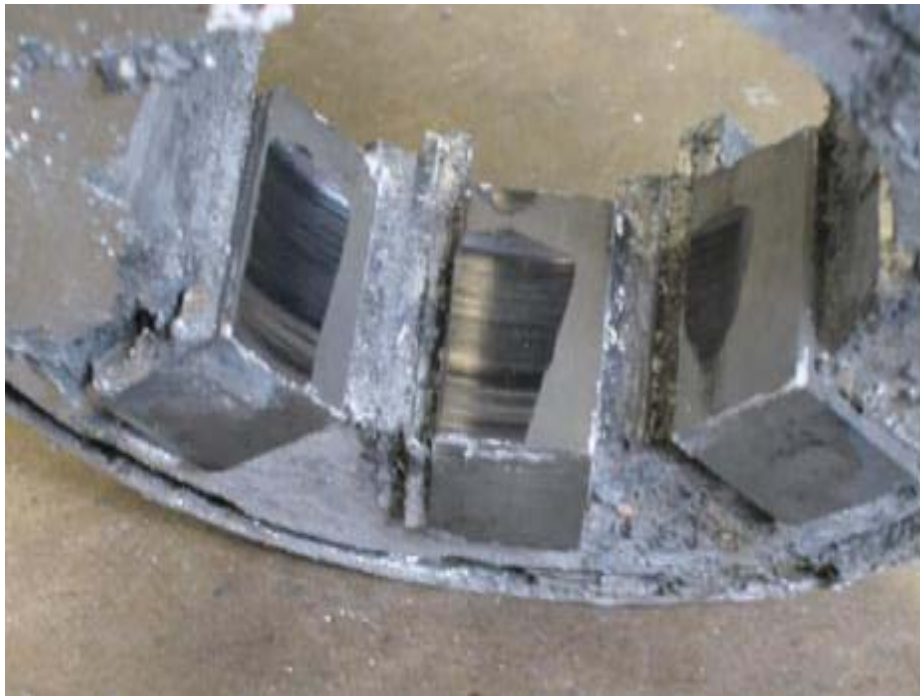
Figure 36 Wearing on Ceramic Insert after Cycle 2 (2hrs at 70% Production Line Tension and 2 hrs at 50% Production Line Tension)
