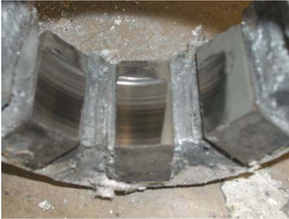
Figure 39 Wearing on Ceramic Insert after Cycle 5 (3 hrs at 50% Production Line Tension)
