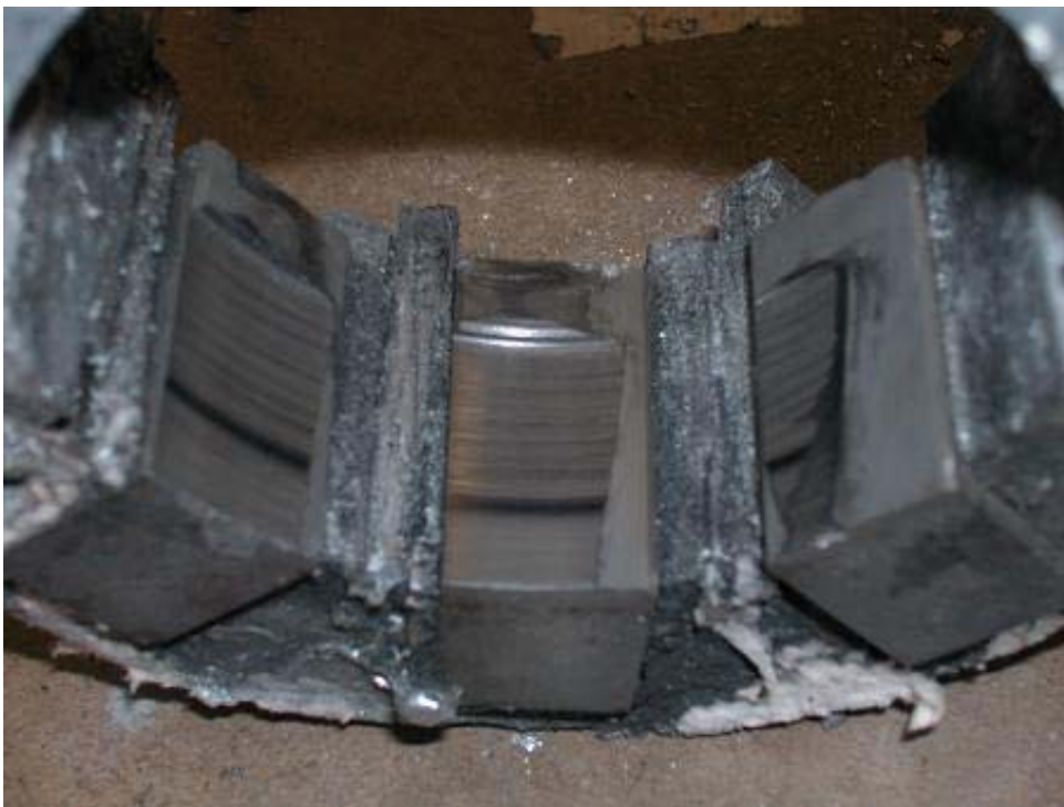
Figure 37 Wearing on Ceramic Insert after Cycle 3 (2 hrs at 50% Production Line Tension)
