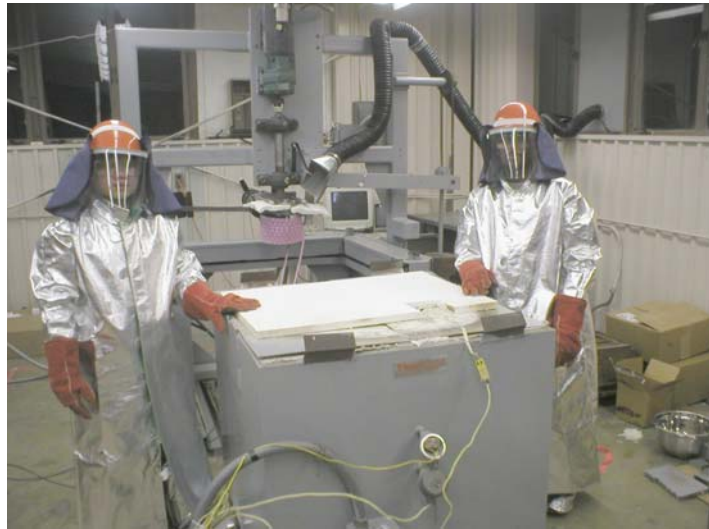
Figure 18 Preheater Wrapped Around the Test Sleeve
