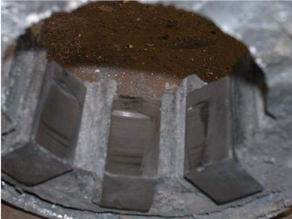
Figure 37 Wearing on Ceramic Insert after Cycle 3 (2 hrs at 50% Production Line Tension)
