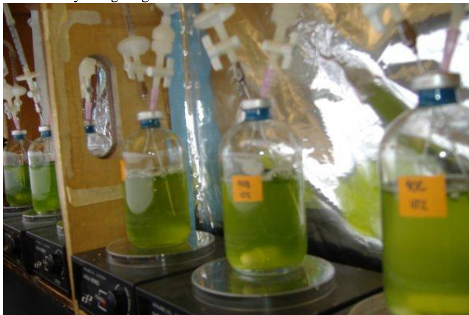
Figure 5. The experimental set-up for evaluation of CO 2 concentration. Glass serum bottles filled with WC medium and sealed with solid stoppers. Two needles were inserted in the stopper to bubble the gas (CO 2 level=0.038%, 3%, 6%, and 12%) through the medium and to provide an exit/sampling point. Light was held constant at 200 \mu\text{mol m}^{-2}\text{s}^{-1} . The medium was stirred continuously using magnetic stirrers.
