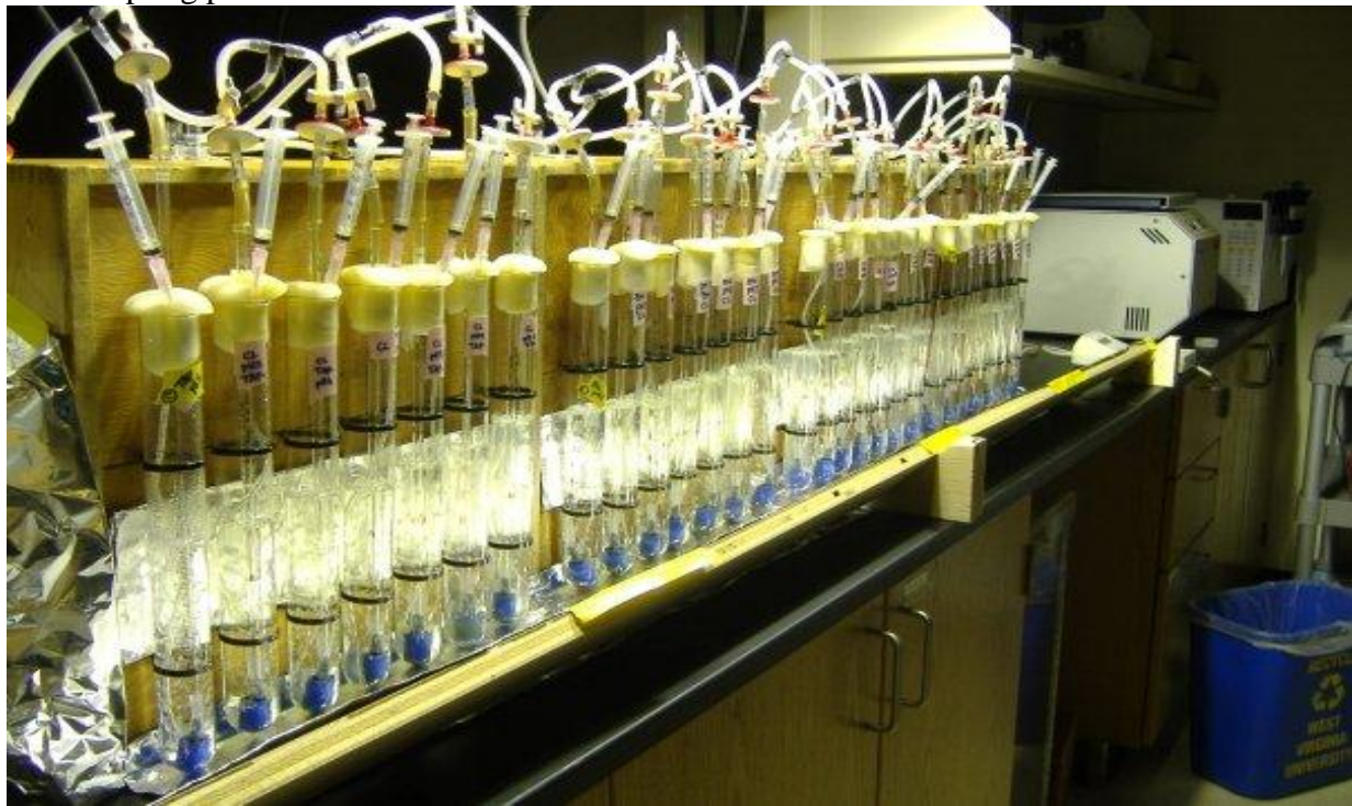
Figure 1. The experimental set-up for evaluation of growth medium and pH (before inoculation). The mouths of the tubes were covered with foam stoppers. Air at 50 mL/min was bubbled through the testing tubes using a pipette to agitate the solution. A syringe provides an exit/sampling point.
