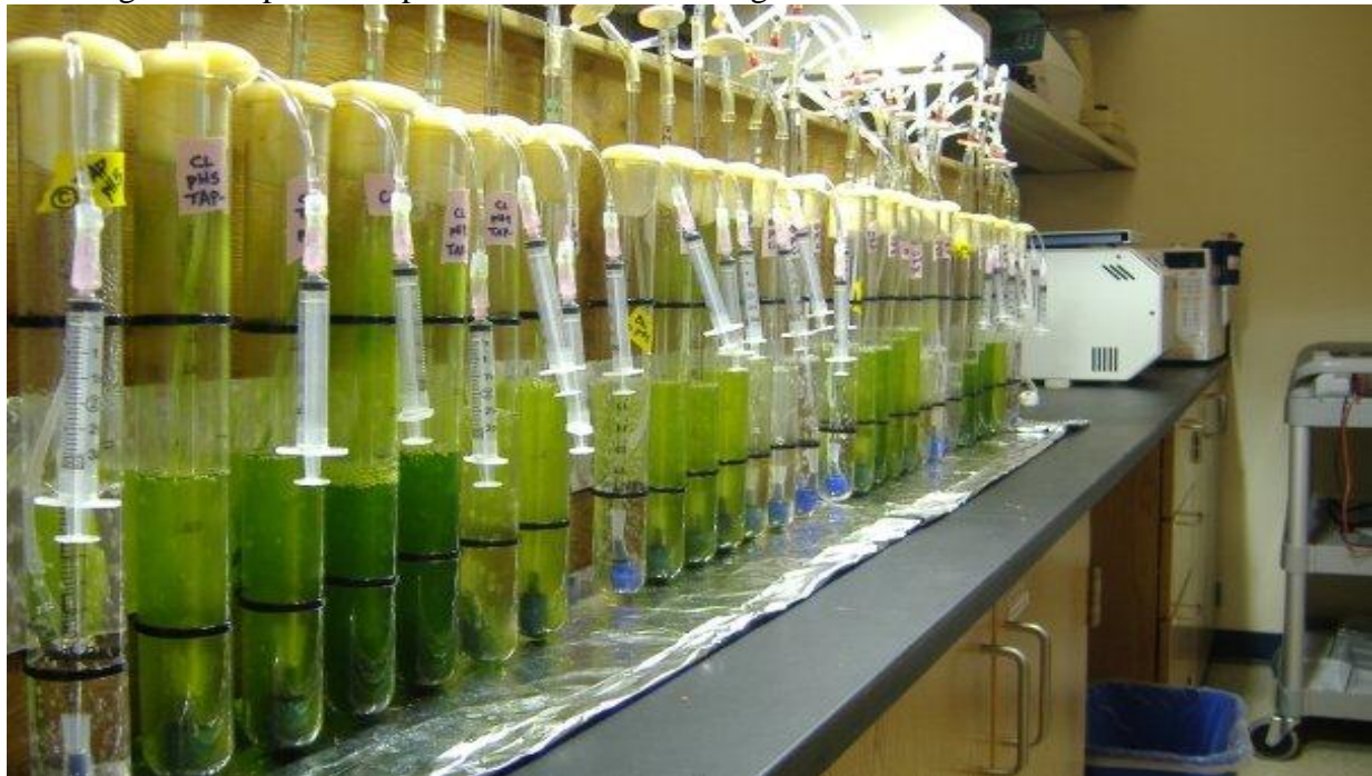
Figure 2. The experimental set-up for evaluation of growth medium and pH (day 5). Visible growth at pH 7 and pH 8. Controls show no growth.
