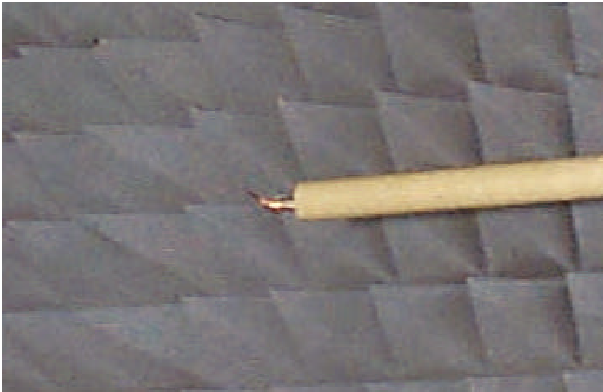
E.7 The transmitting dipole mounted horizontally
