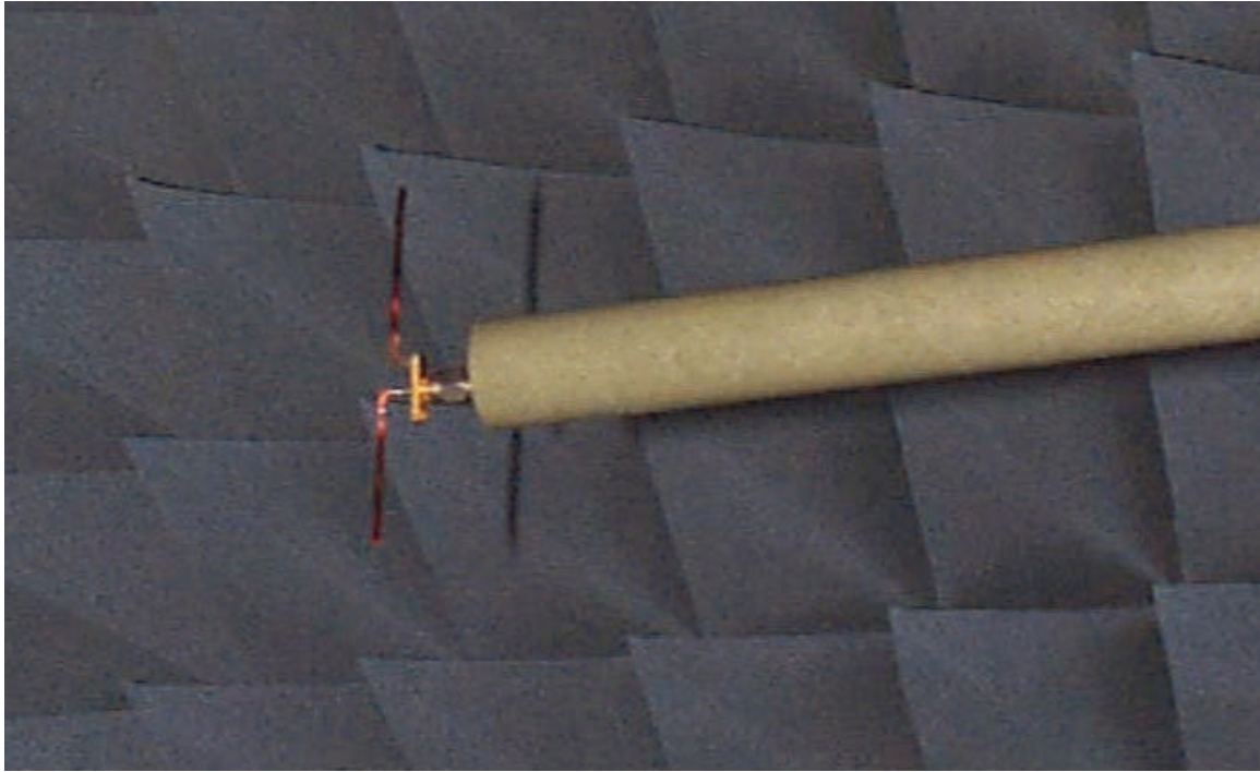
E.8 The transmitting dipole mounted vertically
