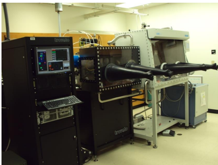
Figure 2.12 Travato Thermal Evaporation System connected to a N 2 filled glovebox.
