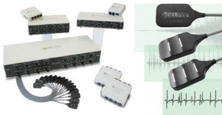
Figure 6: Surface electromyography (EMG) data collection system (Model: Bagnoli, Delsys Inc, Boston, MA, USA) (left) and bi-polar surface electrodes (right).
