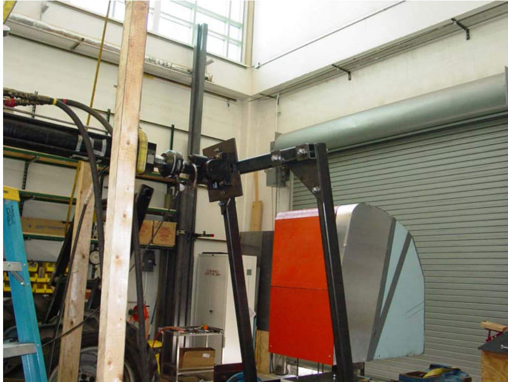
Figure 3-4 SAE J2194 longitudinal loading of Ford-3000 CROPS.
