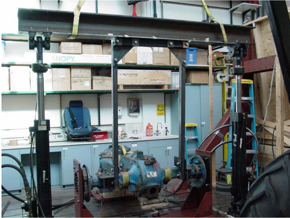
Figure 3-5 SAE J2194 vertical crush loading of Ford-3000 CROPS.
