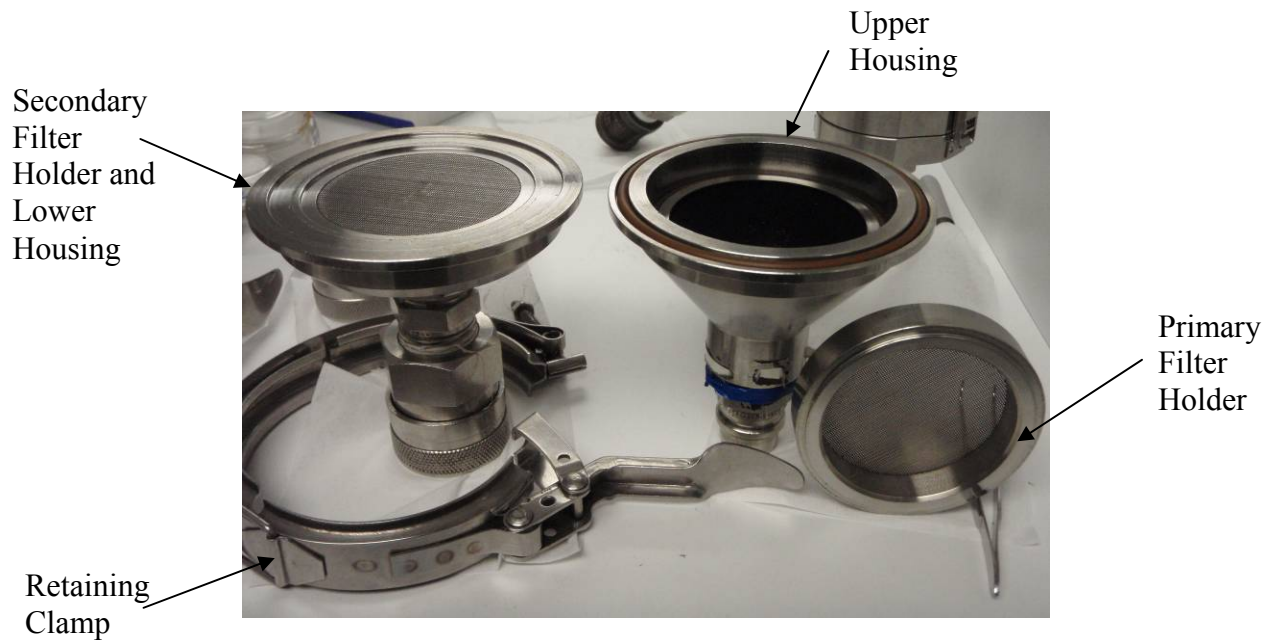
Figure 3- 6 Stainless steel filter housing separated into it's components
