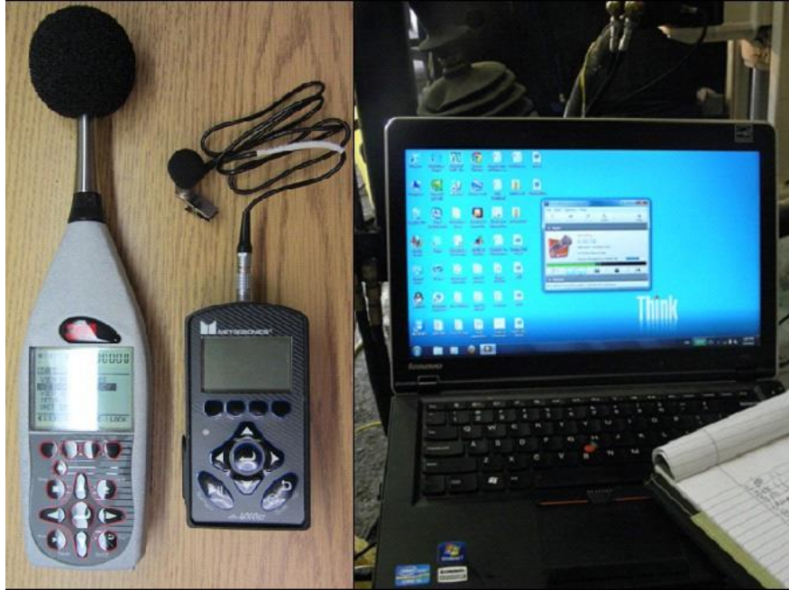
Figure 4.6 Sound Level Meter, Noise Dosimeter, and PC Sound Recording System (left to right) used in noise measurements
