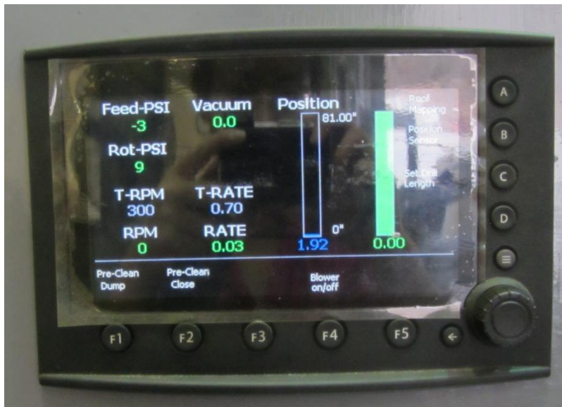
Figure 4.5 Drilling parameters display panel
