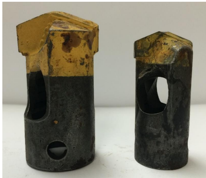
Figure 4.4 Drill bits used in the test (left: 1-3/8-in, right: 7/8-in)
