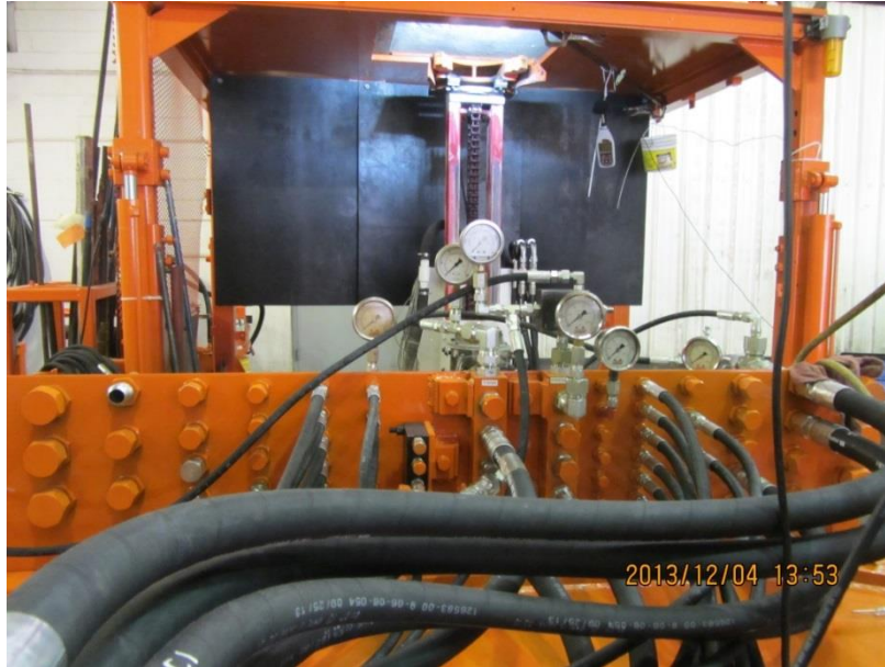
Figure 4.2 Pressure gages of drilling system
