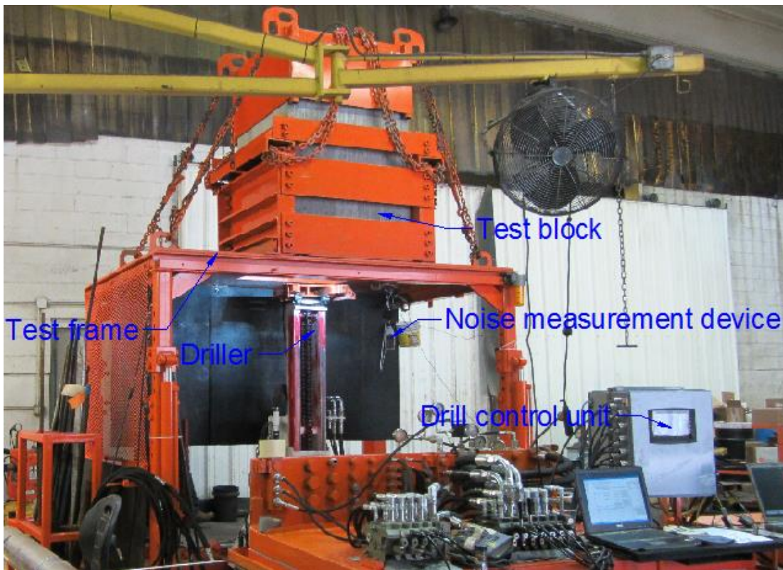
Figure 4.1 Experimental setup of the drilling noise study
