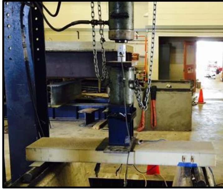
Figure 3.2: Sandwich Bridge deck FRP specimen tested in bending
