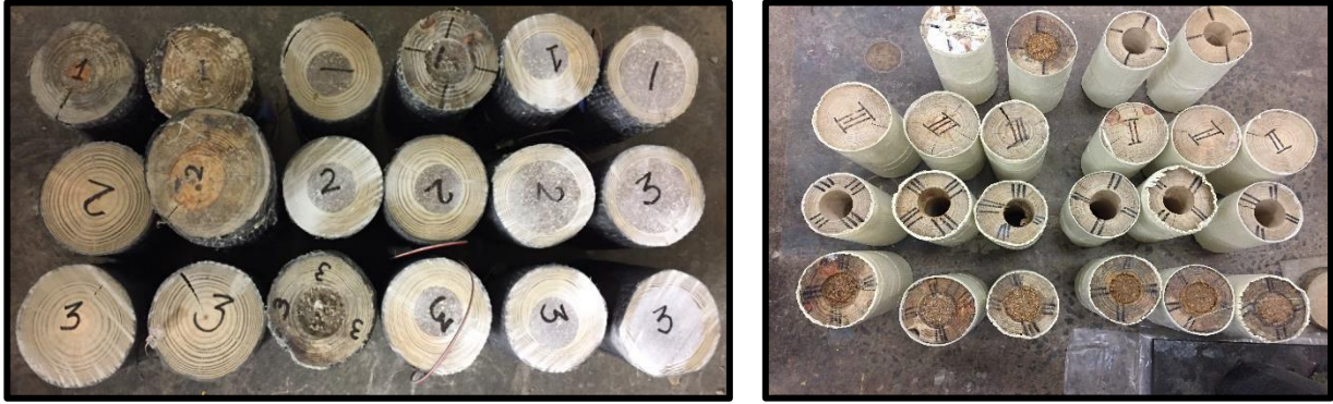
Figure 3.11: Carbon (left) and Glass (right) cylindrical samples ready for testing
