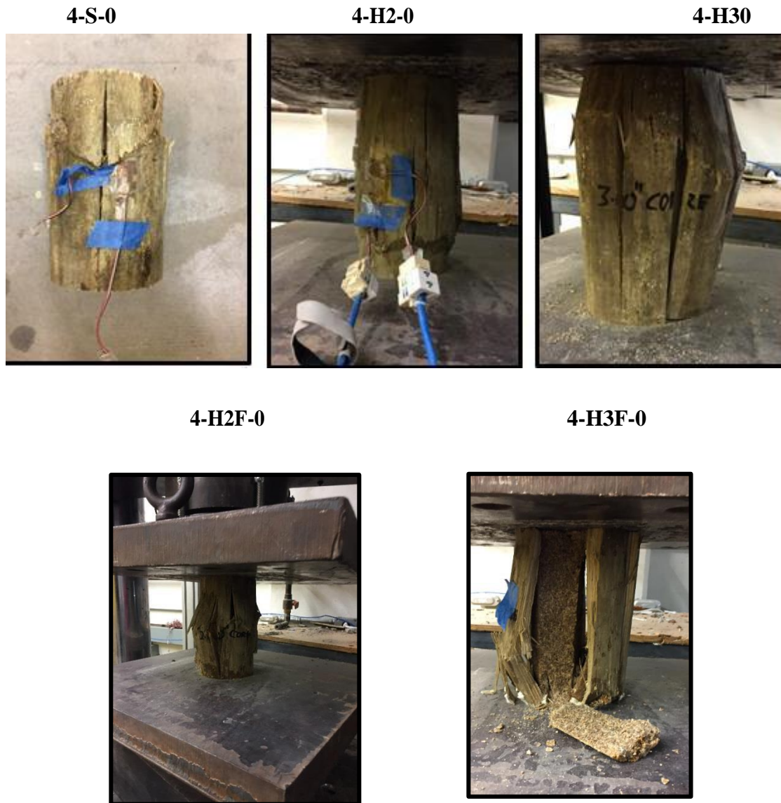
Figure 5.11: Timber cylinders without CFRP wrap and various configurations
