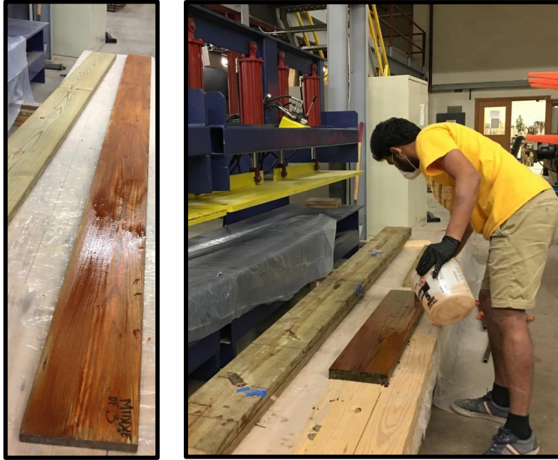
Figure 3.7: Gluing timber members together using Phenolic resin
