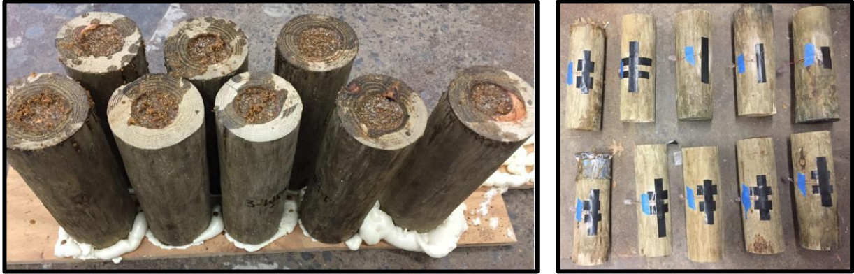
Figure 3.14: Resin filled cylinders along with strain gages attached
