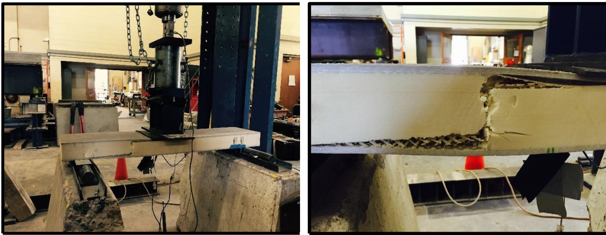
Figure 4.3: FRP Deck tested in 3 point bending (left) and close view of failure region in the deck (right)
