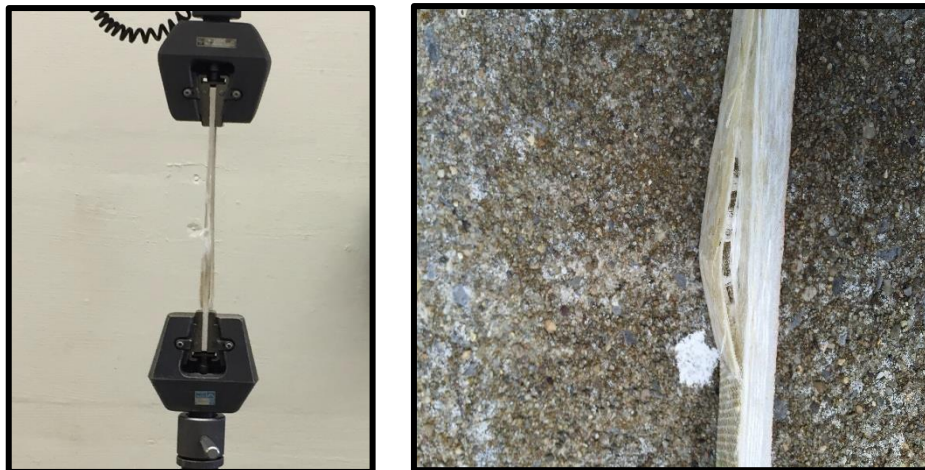
Figure 4.5: Tension coupon with failure at the middle third zone
