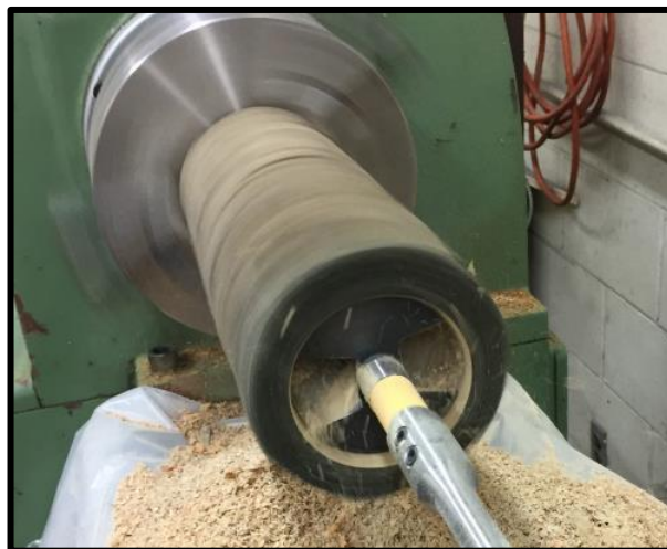
Figure 3.13: Core drilling in a 4.0" cylinder
