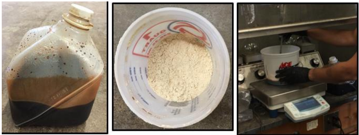
Figure 3.6: Shows the Cascophen and Cascoset and thorough mixing in fume hood
