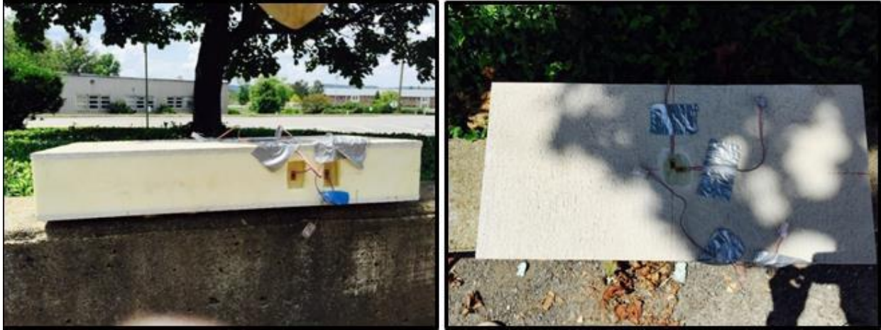
Figure 3.1: Strain gages attached FRP deck specimen1, for shear measurement (Left) and bending stress at center of the span (Right)
