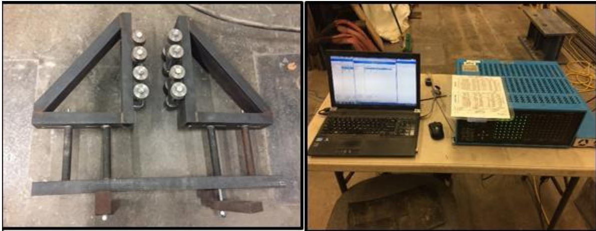
Figure 3.11: Lateral Stabilizers (left) according to ASTM D-198 and Data Acquisition (Right) used during the test
