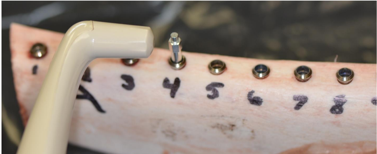
Picture 6: Osstell Mentor probe next to a type 4 SmartPeg on implant number 4 of group A
