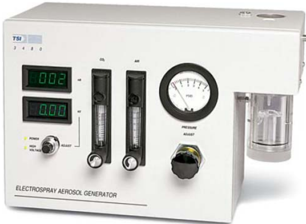
Figure 3-8. TSI Inc. Model 3480 Electro Spray Aerosol Generator [25]
