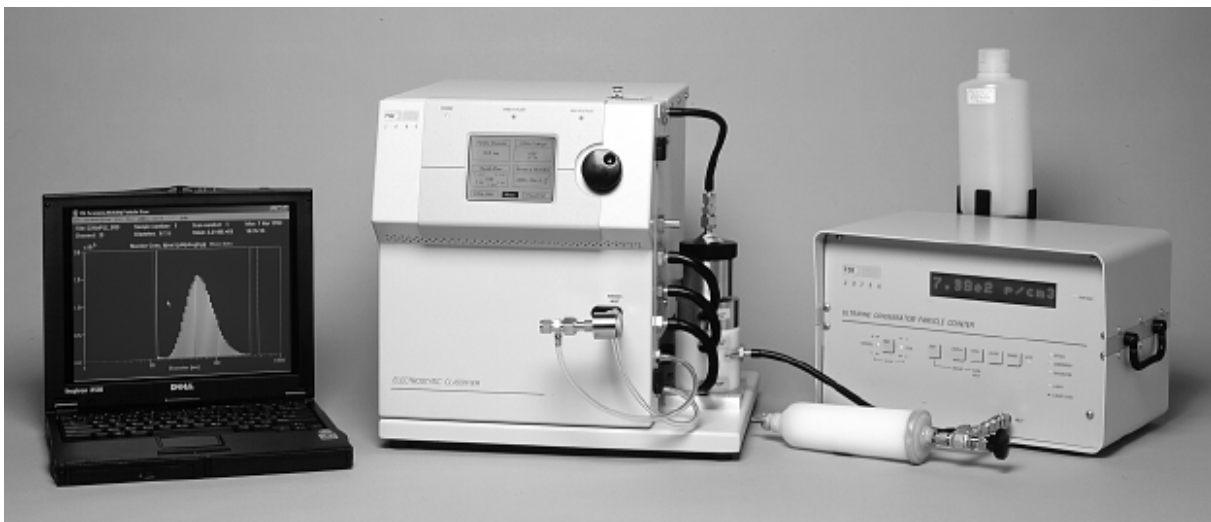
Figure 3-3. SMPS 3936 (Model 3080 Classifier and Model 3025 A CPC) by TSI Inc [24]
