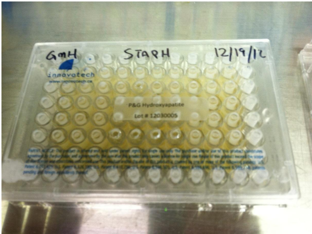
Figure 5 An example of the Calgary Biofilm Device used to simulate a tooth structure.
