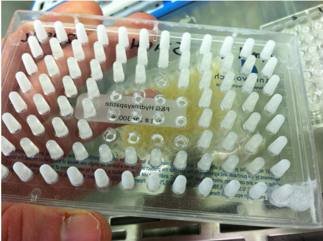
Figure 7 An example of the pegs removed for analysis from the Calgary Biofilm Device.
