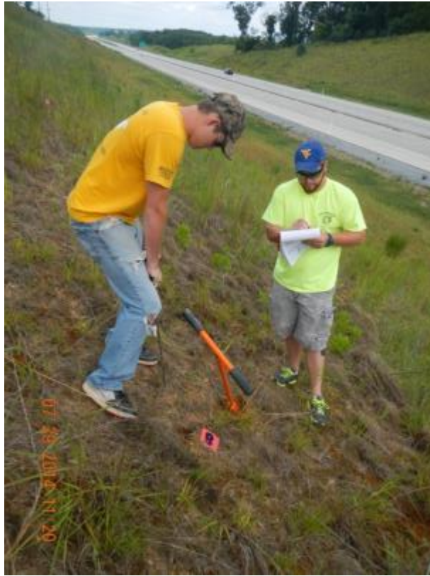
Figure 81: Compaction testing with penetrometer at Route 9 Site 1
