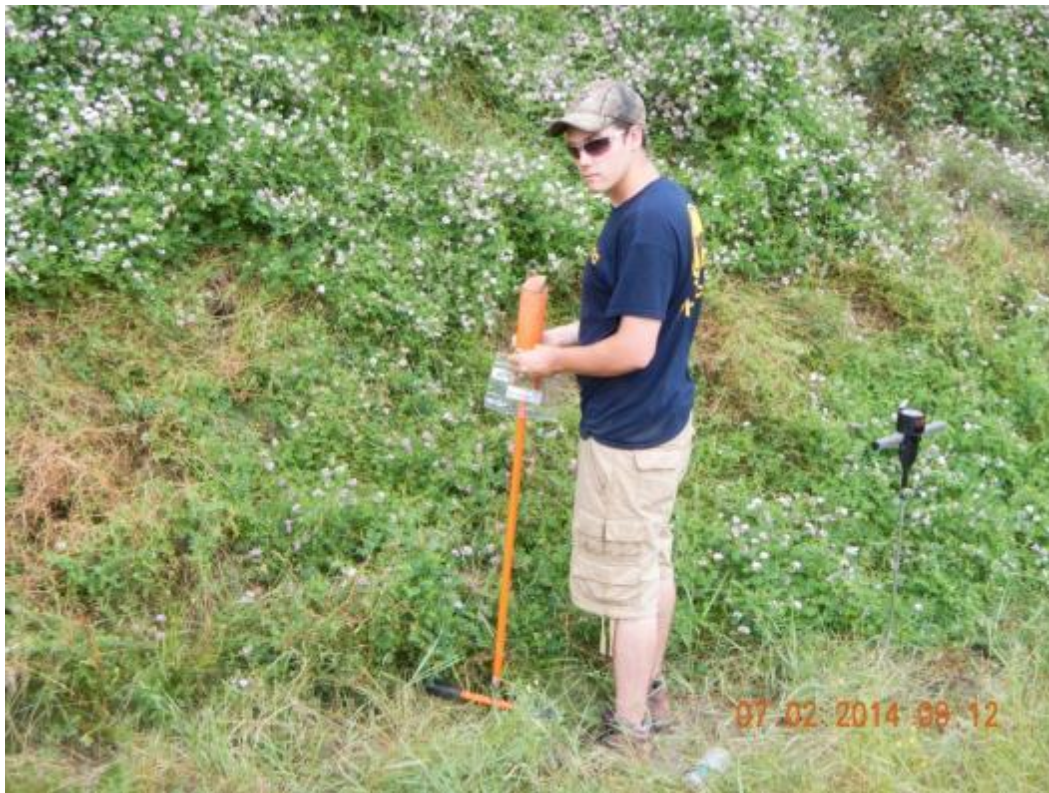
Figure 66: Soil sample collection at Mon-Fayette Expressway Site 1
