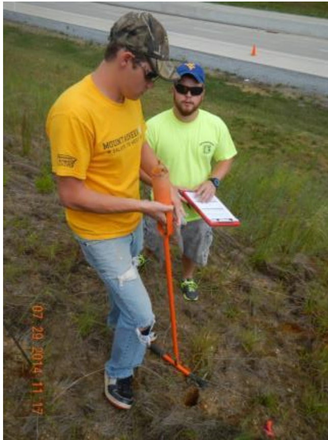
Figure 76: Soil sample collection at Route 9 Site 1
