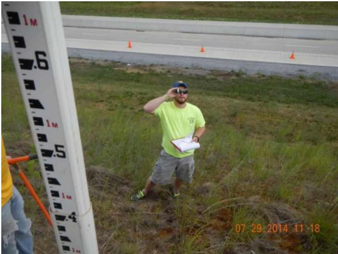
Figure 80: Measurement of slope with clinometer at Route 9 Site 1
