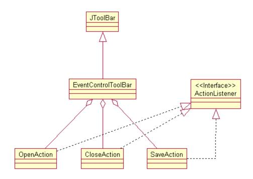
Figure 20 Class Diagram of "EventControlToolBar"
