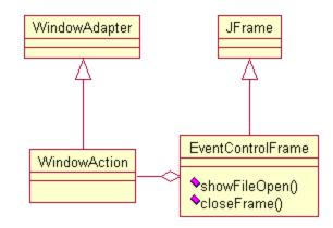
Figure 16 Class Diagram of "EventControlFrame"
