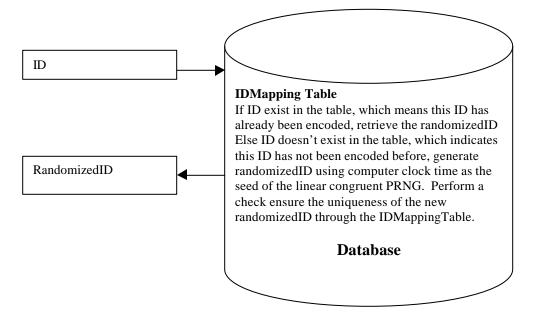
Figure 11 ID Encoding Process Flow Chart
