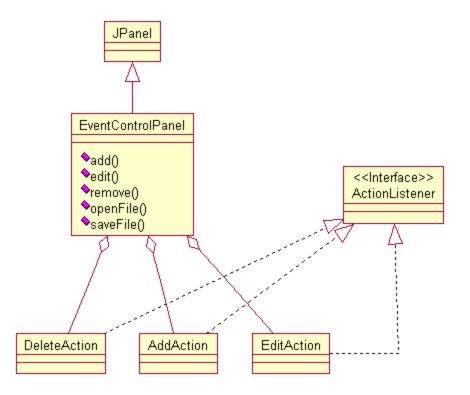
Figure 19 Class Diagram of "EventControlPanel"
