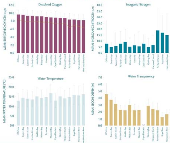
Regions are sorted the same way in all panels (in order of average DO levels, from highest to lowest) so comparisons can be made among parameters. For each region, 90 percent of observations had DO above the orange line. The error bars show +/- one standard deviation among measurements taken in a region to show the magnitude of local, seasonal and annual variability (FOCB 2010).
