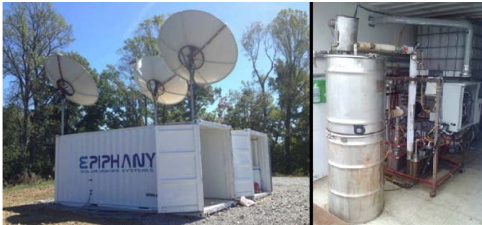
Figure 26: Epiphany's E3H Unit and MKII Distiller at the GH-10 Well Pad
