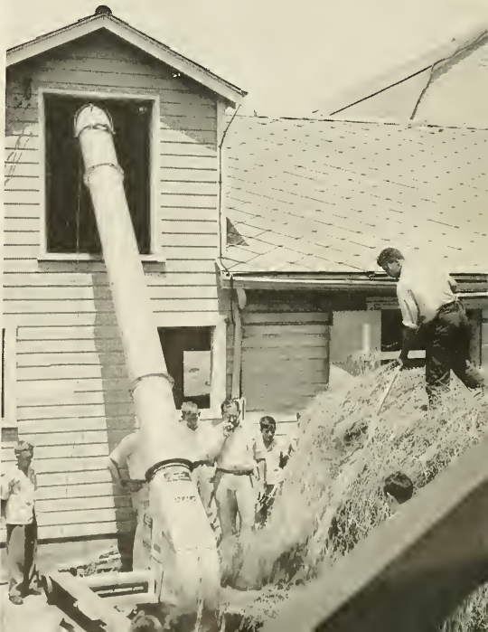
A LONG-HAY blower is demonstrated at WVU Dairy Farm. Field Day visitors see experimental model equipment designed to make farming easier.
