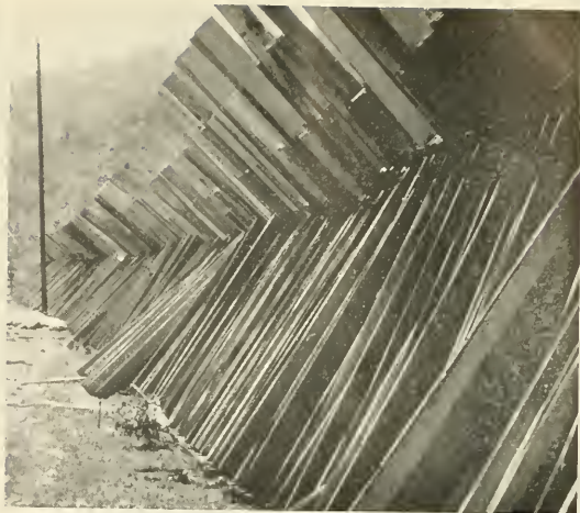
END-STACKING lumber speeds drying and prevents staining.
