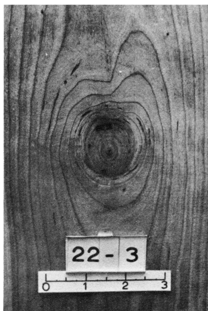
FIGURE 2. A medium, open knot. Wood was sound after the third cut.
