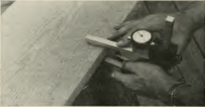
Figure 6. Measurements on the board were made with a micrometer gage to the nearest 1/32 inch.
