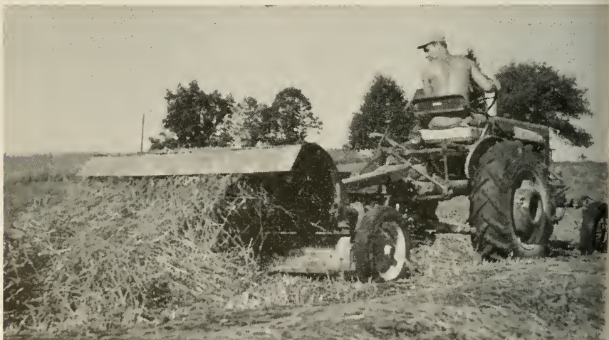
FIGURE 11. Crimper with modified (adjustable) deflector to obtain maximum fluffing.
