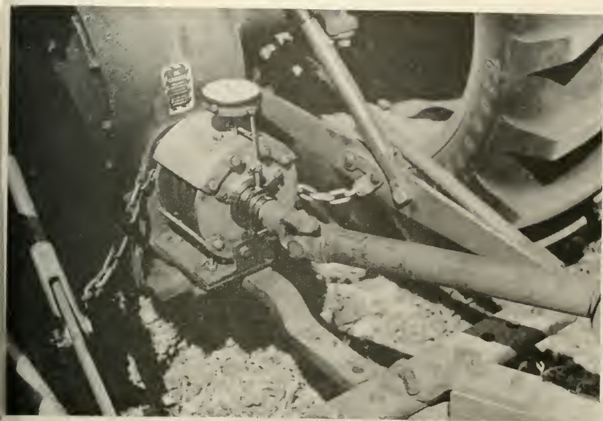
FIGURE 14. PTO dynamometer measuring power requirements of crusher.
