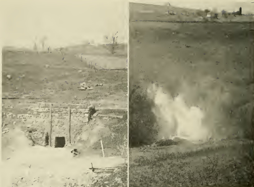
A small and decreasing proportion of the liming materials used in West Virginia is produced locally as burnt lime in permanent kilns (left) and in lime stacks (right). In certain sections where limestone and coal are readily procurable, provided labor is available, these methods of production often prove practicable on a small scale. Much is saved by elimination of heavy freight and trucking costs.
