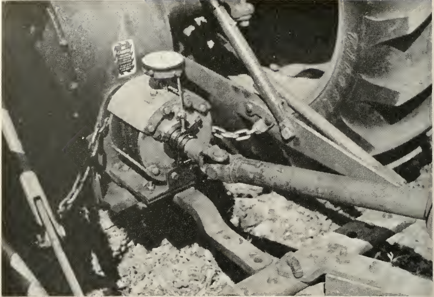
FIGURE 12. The PTO dynamometer mounted on a tractor and coupled to a power-take-off drive.
