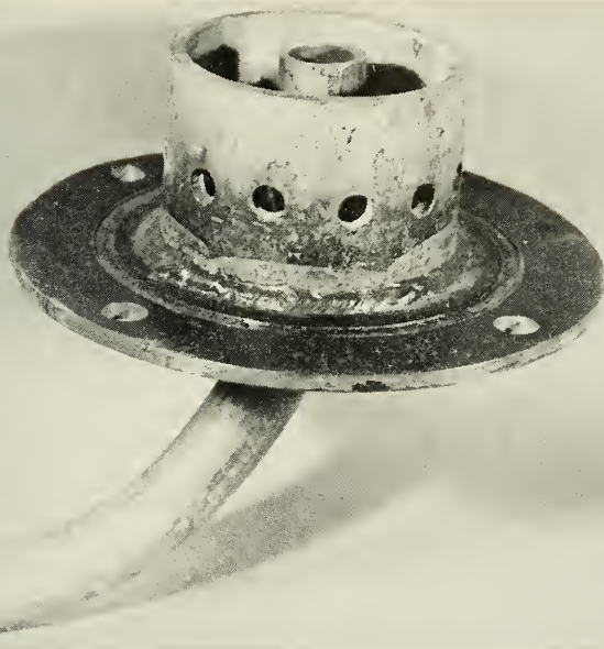
FIGURE 14. A ONE-INCH discharge pipe with lower flange and distribution ring attached.
