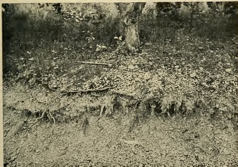
Fig. 7—A road-cut profile in an apple orchard on the Elliber series. Note the high content of chert. A six-inch rule is lying near the bottom of the picture
