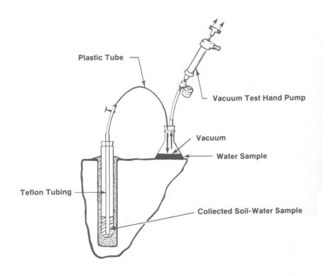
Figure 1. Soil Water Sampler (courtesy, Soilmoisture Equipment Corporation)
