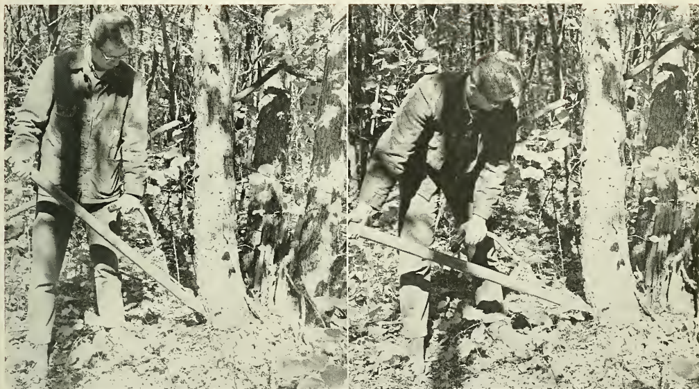
Figure 3. After striking the tree with the injector (left), the unit must be lowered before the handle for releasing the herbicide is depressed (right). If the handle is not lowered, much of the chemical is deposited on the bark above the incision, not on the exposed wood.
