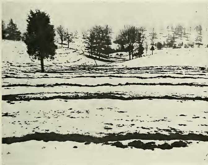
Left: Land treatment which influences the intake of water by the soil or changes the evapotranspiration opportunity offers a limited means of reducing surface runoff or recharging ground water. In an experiment near Moorefield, subsoiling was accomplished by ripping the thinly bedded shale to a depth of 1\frac{1}{2} to 2 feet, making the chisel marks on the contour. Observation of surface runoff and soil moisture changes are being made.
