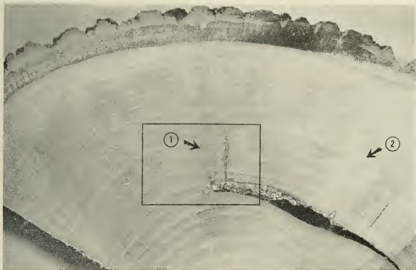
FIGURE 3A. CROSS-SECTIONAL view of blister-shake, in yellowpoplar. Indentations are shown at 1, 2. A frost ring may be seen to the left of the blister-shake in the spring wood of the same annual ring near 1. The boxed area indicates the portion further magnified in Figure 3B.
