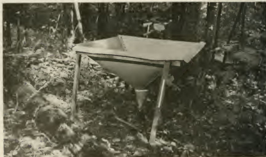
FIGURE 3. A permanent plot with 1,125 oak seedlings per acre in the reproduction class. The seed trap shown is \frac{1}{4} milacre in area and one of a pair maintained under the central oak tree in each permanent plot.
