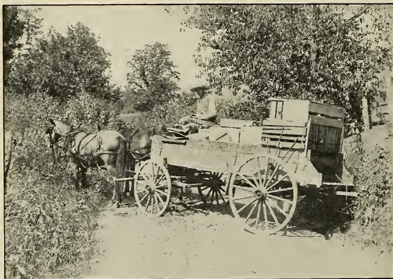
Taking the eggs to market. Note the absence of springs or other shock absorbing arrangement.
