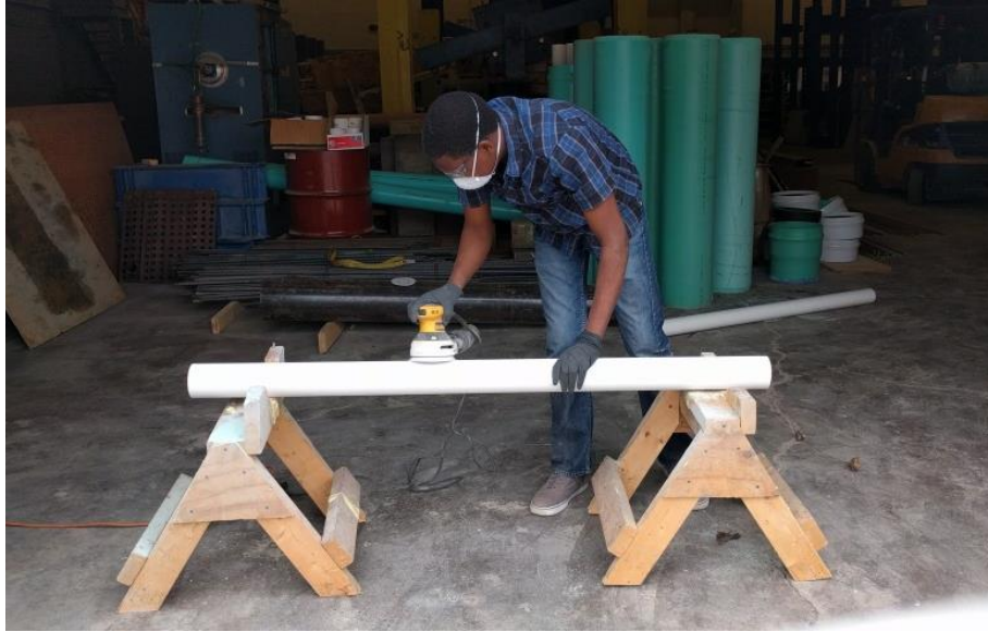
(a) Surface of 3" diameter PVC pipe being sanded
