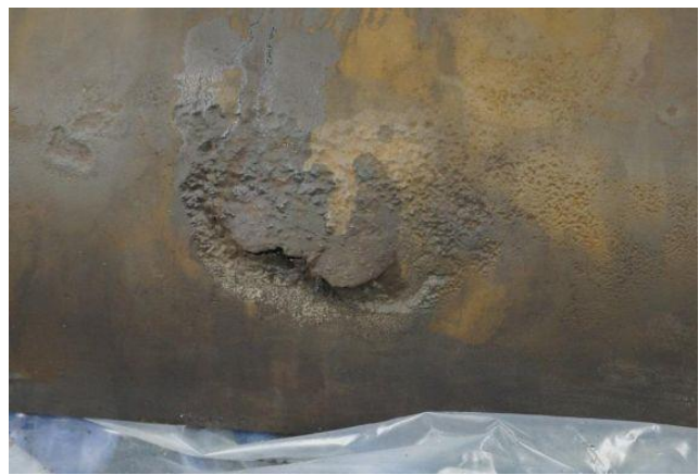
(b) The failed with surrounding insulation and coating removed
