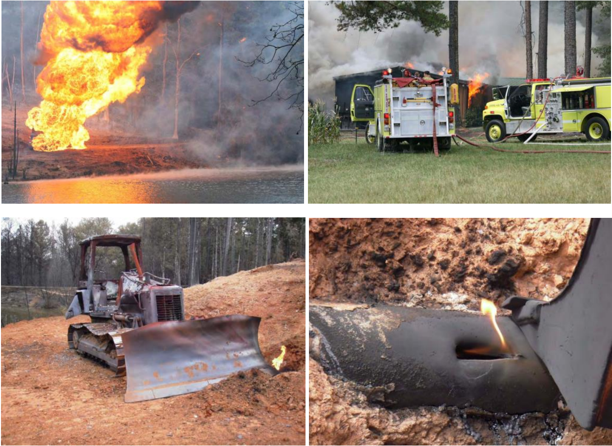
Figure 2-6: Excavation damage explosion (DOT 2011)
