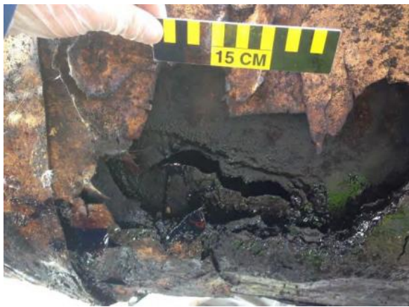
(b) The failed pipe with surrounding insulation and coating
