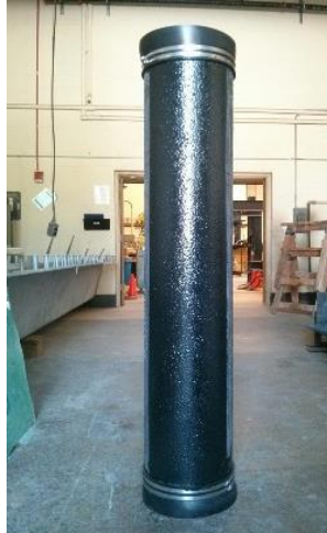
Figure 6-9: 12" diameter GFRP pipe with carbon nanoparticle overlay
