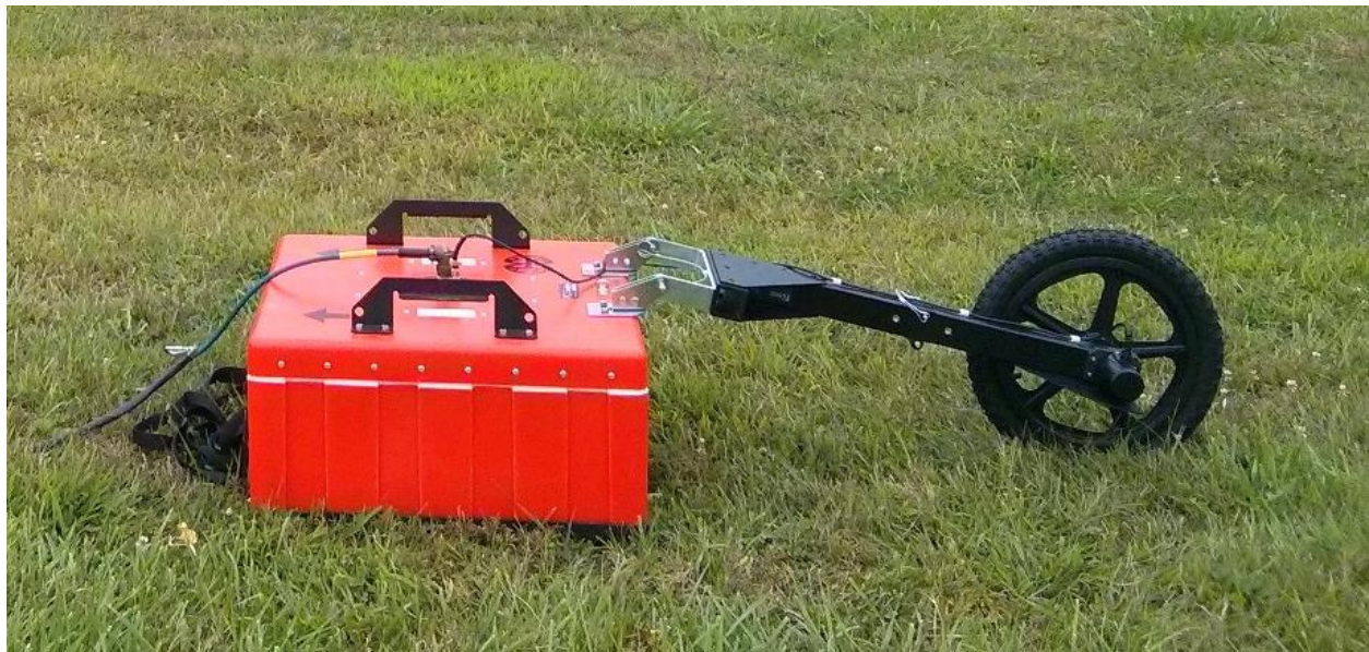
Figure 5-2: 200 MHz GPR antenna with survey wheel
