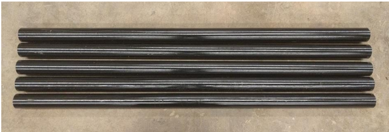
Figure 6-7: The 3" diameter CFRP pipes
