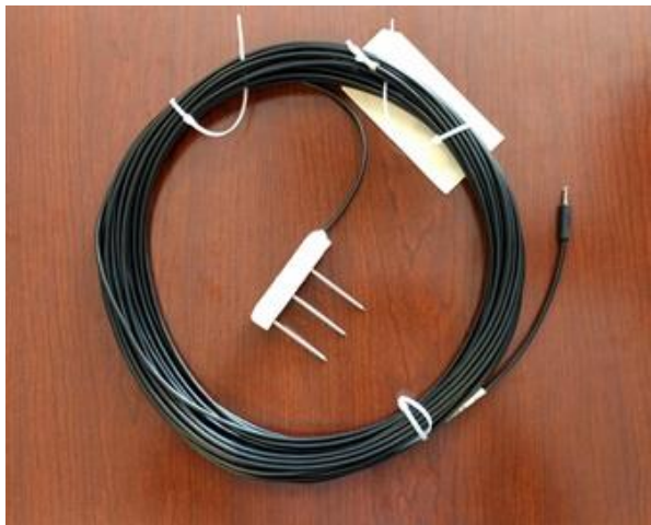
(a) Soil moisture and conductivity sensor
