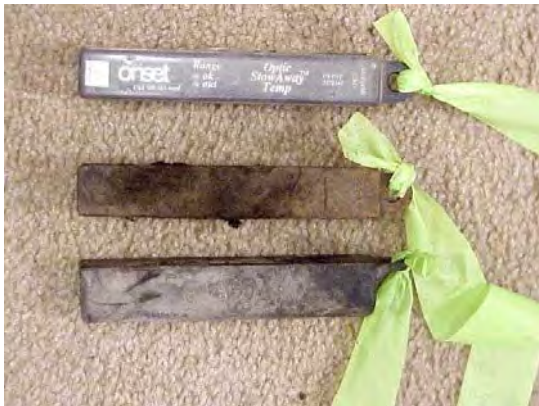
Temperature loggers after retrieval
