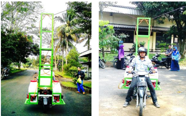
Gambar 7 Mobile sprayer machine (prototipe A) hasil rancangan.
