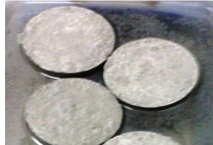
Gambar 7 Sampel Silinder Beton
