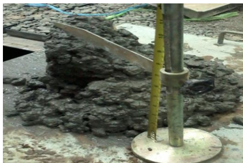
Gambar 8 Uji Slump Campuran Beton
