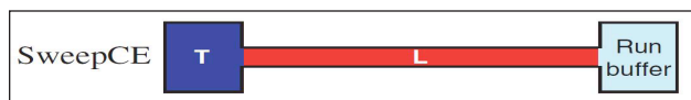
Figure 9, Depiction of initial conditions in SweepCE - No plug is loaded. The intake reservoir contains the target solution. The capillary is prefilled with MRE or other ligand solution.
