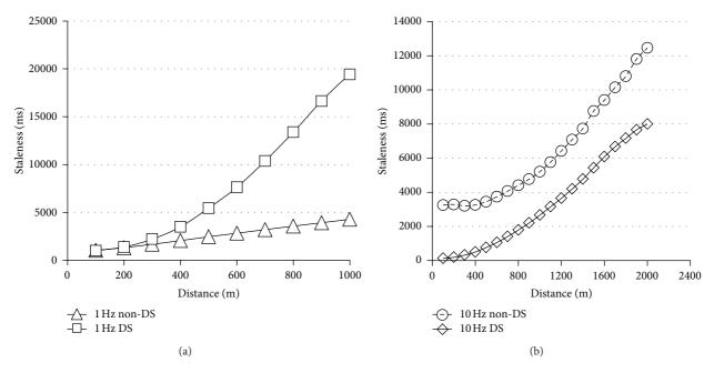
FIGURE 4: Impact of source broadcast rate: *VCAST* versus non-distance-sensitive forwarding. (a) Maximum staleness versus pairwise vehicular distance: p = 1 Hz at 784 nodes. (b) Maximum staleness versus pairwise vehicular distance: p = 10 Hz at 784 nodes.
