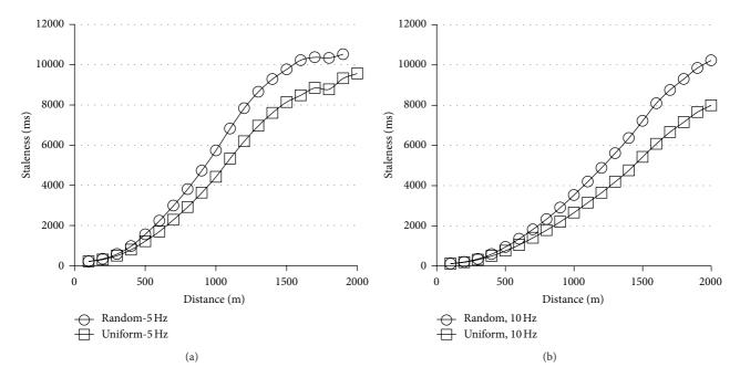
FIGURE 9: Impact of time varying random mobility pattern on *VCAST*: (a) maximum staleness versus pairwise vehicular distance for uniform and random mobility with 784 vehicles, communication range 100 m, source broadcast rate 5 Hz. (b) Maximum staleness versus pairwise vehicular distance for uniform and random mobility with 784 vehicles, communication range 100 m, source broadcast rate 10 Hz.
