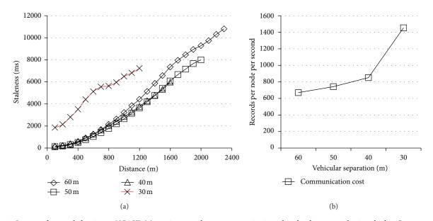
FIGURE 8: Impact of network density on *VCAST*: (a) maximum staleness versus pairwise vehicular distance with 784 vehicles, Communication range 100 m, source broadcast rat 10 Hz, separation 60 m, 50 m, 40 m, and 30 m. (b) Number of vehicular records transmitted by each node per second with 784 vehicles, communication range 100 m, source broadcast rat 10 Hz, separation 60 m, 50 m, 40 m, and 30 m.
