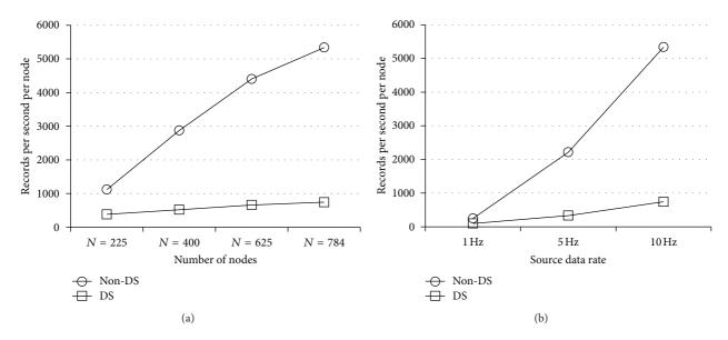
FIGURE 5: Comparison of message complexity: *VCAST* versus non-distance-sensitive forwarding. (a) Number of vehicular records transmitted per second per node at different network sizes for p = 10 Hz and range 100 m. (b) Number of vehicular records transmitted per second per node at different source broadcast rates for 784 nodes and range 100 m.
