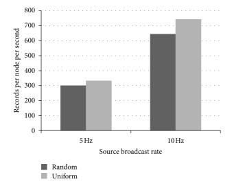
FIGURE 10: Impact of time varying random mobility pattern on *VCAST* (comparison of communication cost): number of vehicular records transmitted by each node per second at 5 Hz and 10 Hz source broadcast rates under uniform and random mobility patterns.
