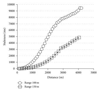
FIGURE 11: Impact of aggregation on *VCAST*: maximum staleness versus vehicle-cell distance with 3600 vehicles, source broadcast rat 10 Hz, communication range 100 m and 150 m.
