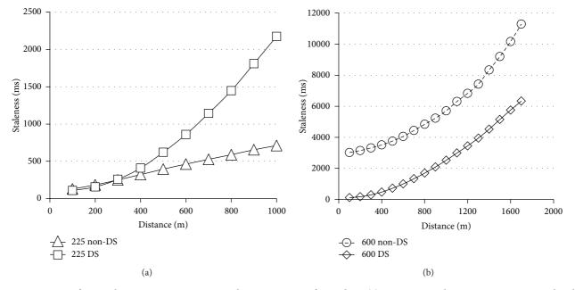
FIGURE 2: Impact of network size: *VCAST* versus non-distance-sensitive forwarding. (a) Maximum staleness versus pairwise vehicular distance: p = 10 Hz at 225 nodes. (b) Maximum staleness versus pairwise vehicular distance: p = 10 Hz at 625 nodes.
