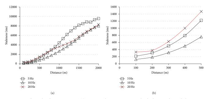
FIGURE 7: Impact of source broadcast rate on VCAST: (a) maximum staleness versus pairwise vehicular distance with 784 vehicles, separation 50 m, communication range 100 m, source broadcast rates of 5 Hz, 10 Hz, and 20 Hz. (b) Zoomed-in version at smaller distances.
