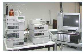
Figure 4. A high performance liquid chromatography, equipped with a diode array detector, a fluorescence detector, and an electrochemical detector (www.aub.edu.lb)
