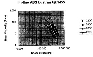
Figure 6. Shear stress vs. shear viscosity
