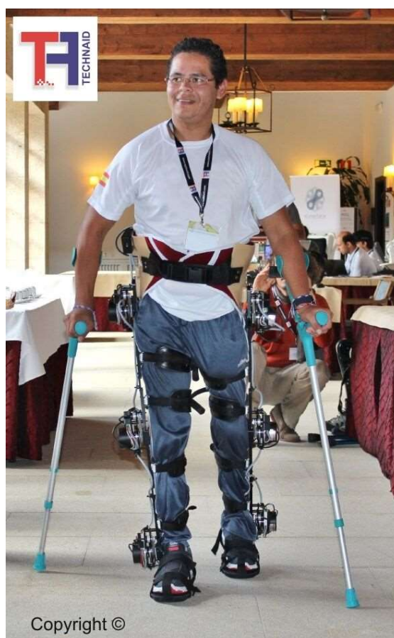
Figura 2. Exo-H2 Exoesqueleto. Exo-H2 by Technaid, S.L.
